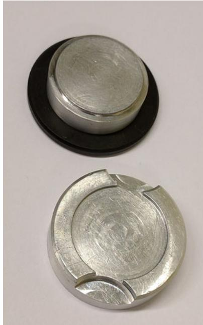
**Fig. 3** Metallic plates made to hold and equally distribute heat and pressure when melting the Parafilm and finalizing the flow cell
