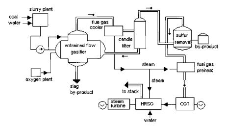
FIGURE 1.3 Wabash integrated coal gasification and combined cycle plant.
