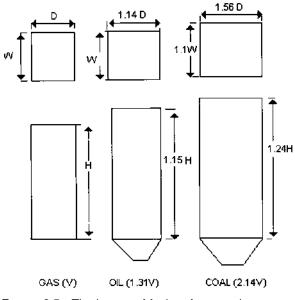
FIGURE 3.5 The impact of fuel on furnace size.
