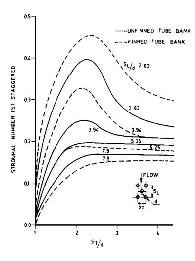
FIGURE 8.25b Strouhal number for staggered bank of tubes.
