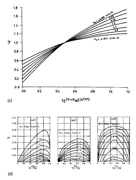
**FIGURE 8.1c,d** (c) Correction factor for emissivity of water vapor. (d) Correction term due to presence of water vapor and carbon dioxide. (From Ref 1.)
