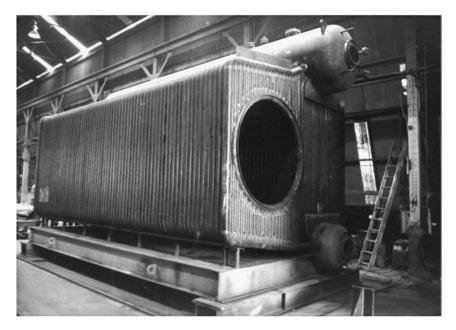
**FIGURE 3.2** Completely water-cooled furnace design. (Courtesy of ABCO Industries, Abilene, TX.)
