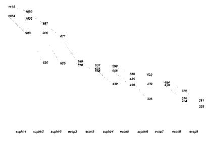
**FIGURE 1.17b** Temperature profiles and performance of the HRSG.
