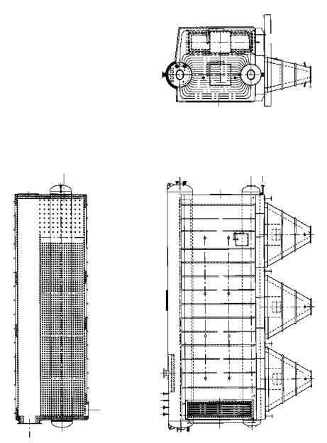
**FIGURE 2.15** Waste heat boiler in carbon black plant. (Courtesy of ABCO Industries, Abilene, TX.)
