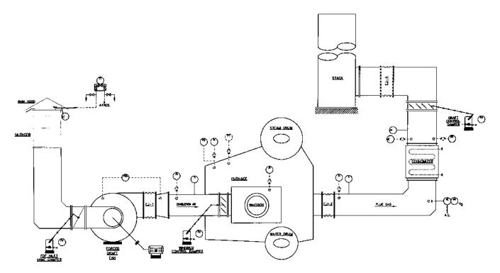
FIGURE 3.15a Scheme of boiler controls-gas side. (Courtesy of ABCO Industries, Abilene, TX.)
