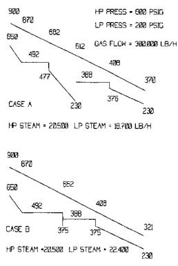
Figure 8.15 Optimizing temperature profiles.
