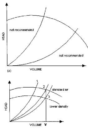
Curve 1 is the actual operating curve while curve 2 is the estimated.Operating at point 1 is not recommended.
