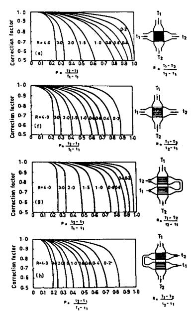
FIGURE 8.10 Crossflow correction factors (From Refs. 1 and 2).
