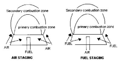
FIGURE 4.12 Staging of fuel and air in burners.
