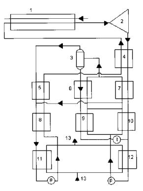
**FIGURE 1.4** Kalina cycle scheme at Canoga Park, CA. 1, HRVG; 2, turbine; 3, flash tank; 4, final preheater; 5, HP preheater; 6, second recuperator; 7, vaporizer; 8, HP preheater; 9, first recuperator; 10, LP preheater; 11, HP condenser; 12, LP condenser; 13, cooling water; t, throttling device; p, pump.
