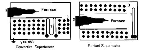
**FIGURE 3.17** Location of convective and radiant superheater. 1, Superheater; 2, burner; 3, screen evaporator.
