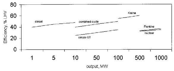
FIGURE 1.1 Efficiency of typical power systems.
