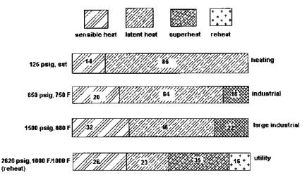
FIGURE 3.6 Distribution of energy in boilers as a function of steam pressure.
