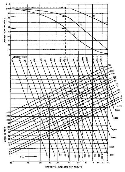
**FIGURE 9.3a** Viscosity corrections. (Courtesy of Hydraulic Institute/Gould Pump Manual.)
