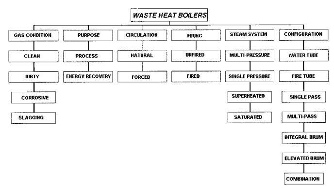
FIGURE 2.1 Classification of waste heat boilers.
