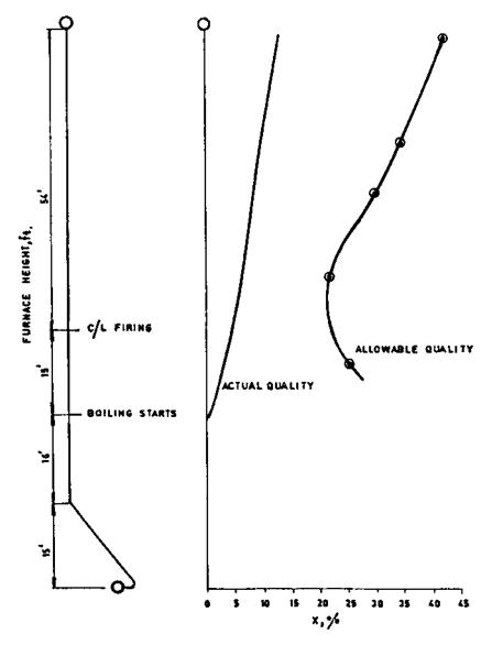
FIGURE 7.13 Actual quality vs. allowable quality along furnace height.
