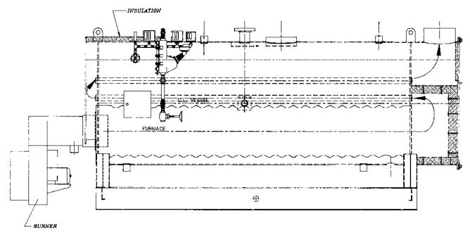
FIGURE 3.3b Fire tube boiler—dryback design.
