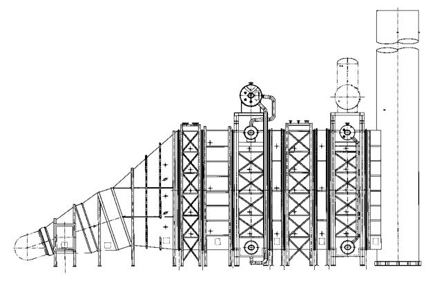
FIGURE 1.13 Multipressure supplementary-fired HRSG.
