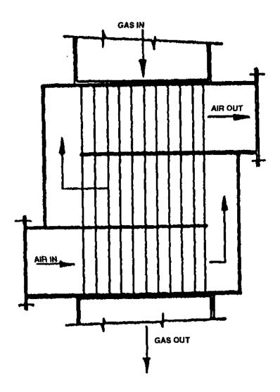
FIGURE 8.9 Tubular air heater.
