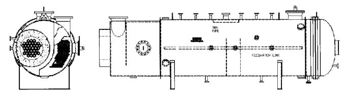
FIGURE 2.5 Waste heat boiler for sulfur recovery plant. (Courtesy of ABCO Industries, Abilene, TX.)
