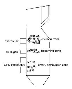
FIGURE 4.15 Reburning and NOx reduction.
