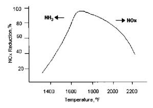
FIGURE 4.4 Range of temperatures for SNCR operation.
