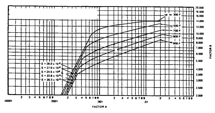
FIGURE 5.4 Factor *B* for use in external pressure calculation (SA 178A, SA 192 tubes) [9].
