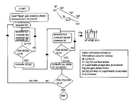
FIGURE 2.17 Logic used for evaluating HRSG performance.
