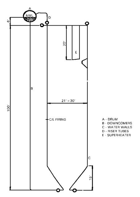
**FIGURE 7.4** Scheme of natural circulation boiler showing furnace, drum, riser, and downcomer circuits.
