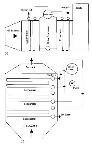
**FIGURE 2.12** HRSGs with different type of circulation systems: (a) Natural circulation, (b) forced circulation. (c) Once-through.
