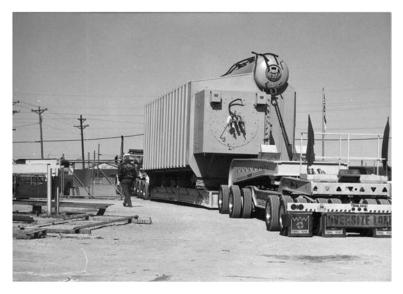
**FIGURE 1.5** Packaged steam generator with completely water-cooled furnace. (Courtesy of ABCO Industries, Abilene, TX.)
