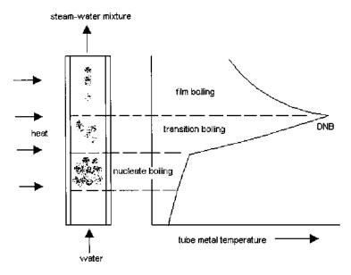
FIGURE 3.13 Boiling process and DNB in boiler tubes.
