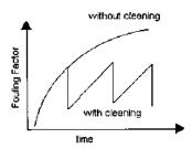
FIGURE 2.16 Fouling in waste heat boilers versus time.
