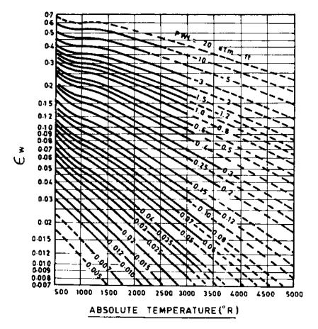
FIGURE 8.1b Emissivity of water vapor. (From Ref 1.)
