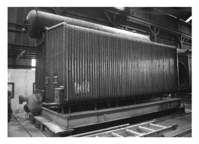
FIGURE 4.2 Water-cooled furnace. (Courtesy of ABCO Industries, Abilene, TX.)
