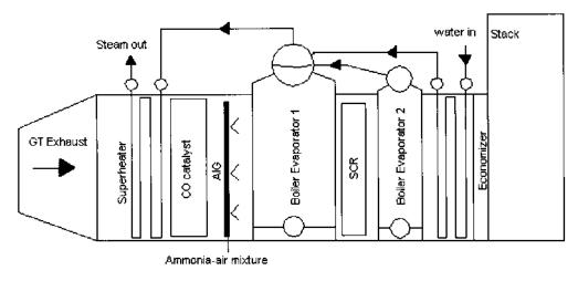
FIGURE 4.7 HRSG showing location of NOx (SCR) and CO catalysts.
