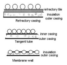
**FIGURE 3.10** Furnace construction—membrane wall, tangent tube, and refractory wall.
