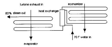
FIGURE 2.13 HRSG used in oil field applications.
