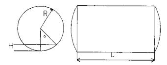
FIGURE 5.5 Partial volume of water in boiler drum.
