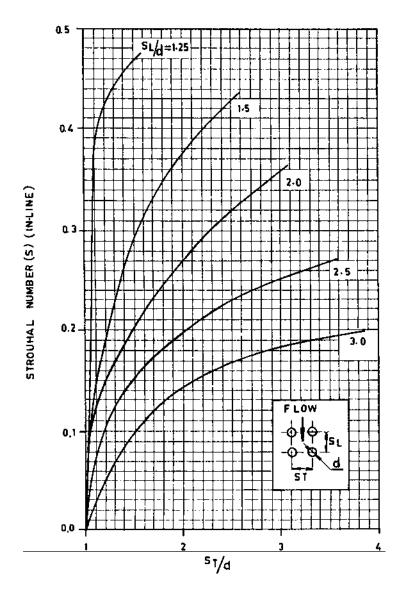
FIGURE 8.25a Strouhal number for in-line bank of tubes.
