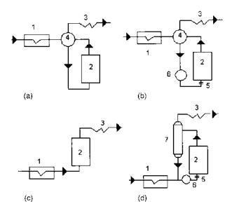
**FIGURE 3.4** Boiler circulation methods. (a) Natural; (b) forced circulation; (c) once-through; (d) once-through with superimposed circulation. 1, Economizer; 2, furnace; 3, superheater; 4, drum; 5, orifice; 6, circulating pumps; 7, separator.
