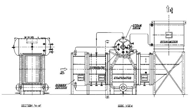
FIGURE 2.3 Water tube waste heat boiler with superheater and economizer. (Courtesy of ABCO Industries, Abilene, TX.)
