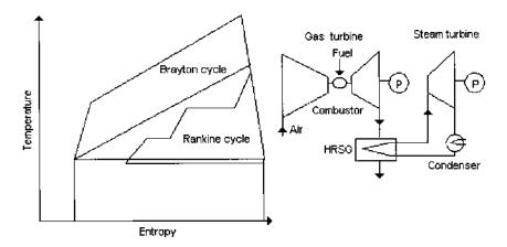
FIGURE 1.9a Combined cycle system showing the Brayton–Rankine cycle.
