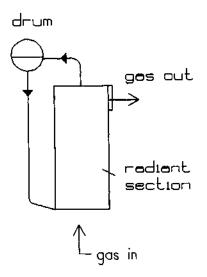
Figure 8.2 Radiant furnace in a water tube boiler.
