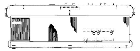
FIGURE 3.19a Inverted loop superheater arrangement. (Courtesy of ABCO Industries, Abilene, TX.)
