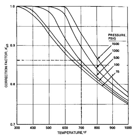
FIGURE 7.1 Correction factors for superheat.
