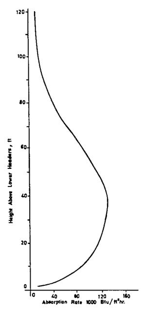
FIGURE 7.11 Typical heat absorption rates along furnace height.
