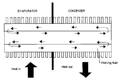
FIGURE 3.28 Arrangement of a heat pipe.
