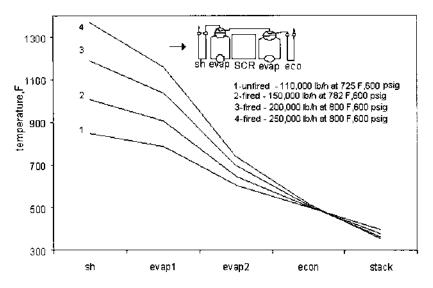
**FIGURE 4.8** HRSG gas temperature profiles as a function of steam generation. sh, superheater; econ, economizer; evap, evaporator.
