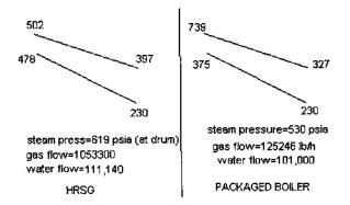
FIGURE 3.25 Economizer temperature pick-up in boiler versus HRSG.
