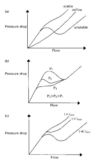
**FIGURE 7.18** Effect of (a) orifice size, (b) pressure, and (c) inlet subcooling on the stability of two-phase boiling circuits.
