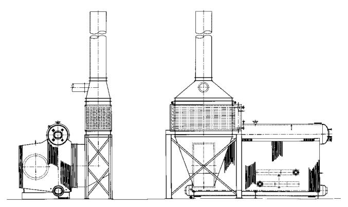
FIGURE 3.23a Economizer in a packaged boiler. (Courtesy of ABCO Industries, Abilene, TX.)
