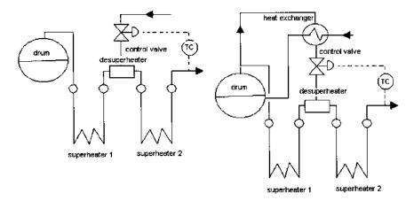
FIGURE 3.18 Steam temperature control methods.
