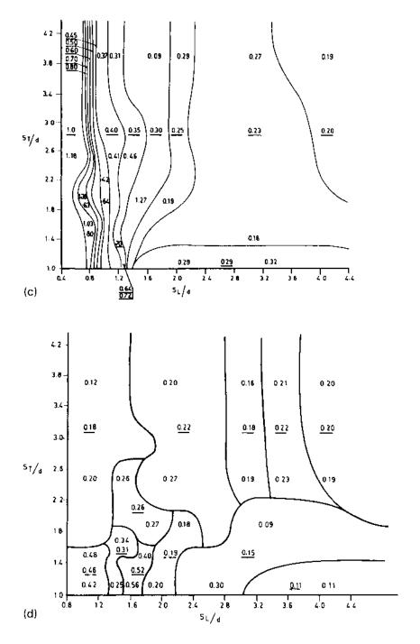
**FIGURE 8.25c,d** Strouhal number (c) for staggered bank of tubes (top), (d) for inline bank of tubes (bottom).
