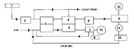
**FIGURE 2.10** Steam reforming process in hydrogen plants. 1, natural gas; 2, sulfur removal; 3, reformer; 4, reformed gas boiler; 5, flue gas boiler; 6, shift converter; 7, air preheater; 8, air; 9, CO<sub>2</sub> removal and methanation; 10, Pressure Swing Adsorption (PSA); 11, H<sub>2</sub> product; 12, stack; 13, CO<sub>2</sub> by-product.
