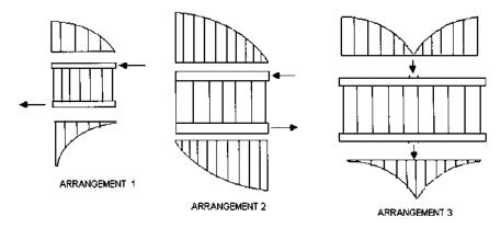
FIGURE 3.21 Flow nonuniformity due to header arrangements.
