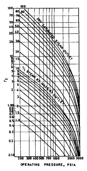
**FIGURE 7.8** Thom's two-phase multiplication factor for acceleration loss. (See Refs. 11, 15, and 16.)
