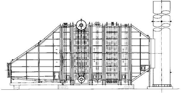
FIGURE 1.10 Unfired HRSG in a gas turbine plant.
