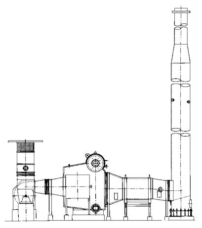
**FIGURE 3.1** Package water tube boiler. (Courtesy of ABCO Industries, Abilene, TX.)
