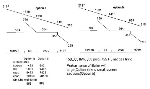
**FIGURE 3.20** Results from boiler program showing effect of screen section on superheater performance. Option a: More screen rows; option b: fewer screen rows.
