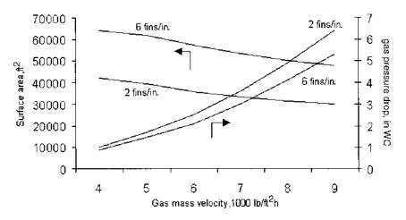
**FIGURE 8.8** Effect of fin geometry on HRSG surface area and gas pressure drop.
