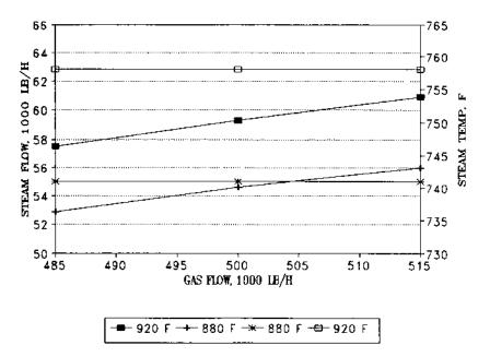
FIGURE 8.18 HRSG performance as a function of gas flow and temperature.
