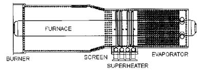
FIGURE 1.14a Furnace-fired HRSG arrangement.
