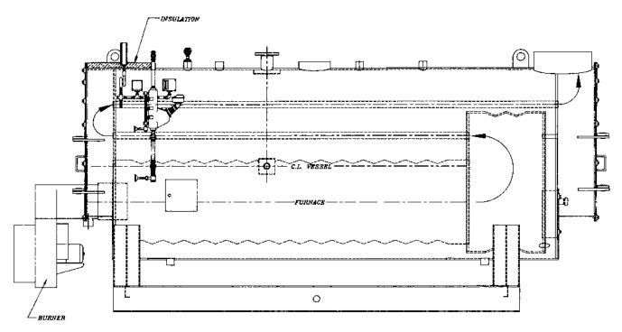
FIGURE 3.3a Fire tube boiler—wetback design.
