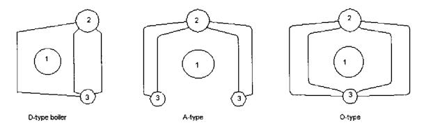
FIGURE 3.7 A-, D-, and O-type boiler configurations. 1, Burner; 2, steam drum; 3, mud drum.
