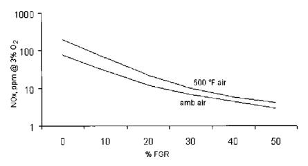
FIGURE 4.13 NOx versus flue gas recirculation.
