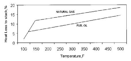
FIGURE 3.29 Efficiency improvement in oil and gas firing using a condensing exchanger.
