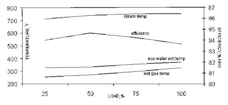
FIGURE 3.24 Boiler performance versus load.
