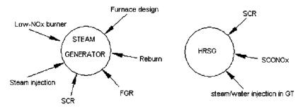
FIGURE 4.3 Options for NOx removal in boilers and HRSGs.
