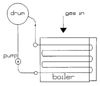
FIGURE 7.5 Scheme of forced circulation boiler.
