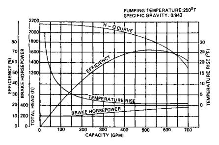
**FIGURE 9.4** Typical characteristic curve of a multistage pump also showing temperature rise versus capacity.
