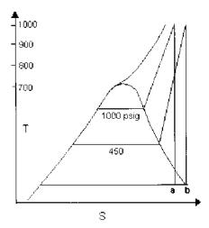
FIGURE 1.6 T–S diagram showing expansion of steam.
