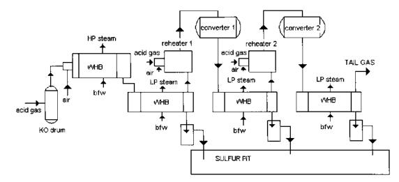
FIGURE 2.4 Claus process for sulfur recovery.
