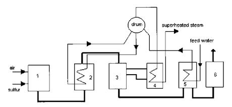
**FIGURE 2.9** Scheme of a sulfuric acid plant. 1, sulfur combustion furnace; 2, waste heat boiler; 3, contact apparatus; 4, superheater; 5, economizer; 6, absorption tower.
