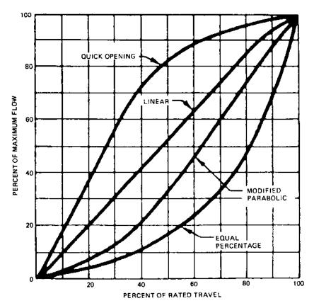
FIGURE 7.2 Typical control valve characteristics.
