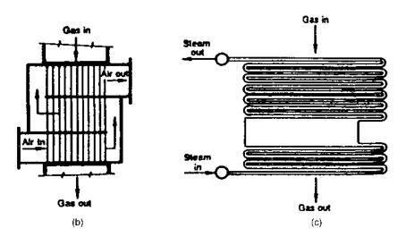
**FIGURE 8.24** Crossflow of gas over tube bundles. (a) Water tube boiler design; (b) air heater; (c) superheater.
