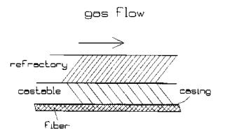
FIGURE 8.21 Arrangement of hot casing.
