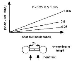
FIGURE 3.11 Relating fin tip temperature to heat flux in membrane wall furnace.
