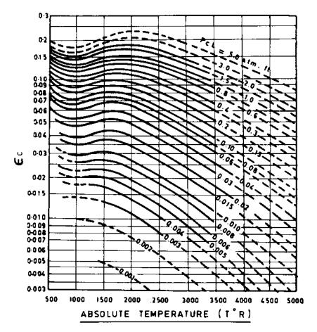
FIGURE 8.1a Emissivity of carbon dioxide. (From Ref 1.)
