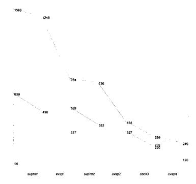
**FIGURE 8.16b** Fresh air fired temperature profile.
