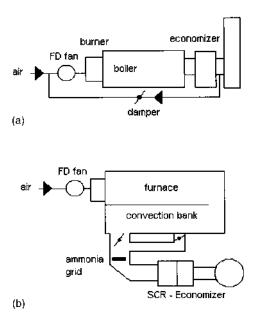
**FIGURE 4.6** Gas bypass system in boiler using (a) FGR and (b) SCR methods for NOx control.
