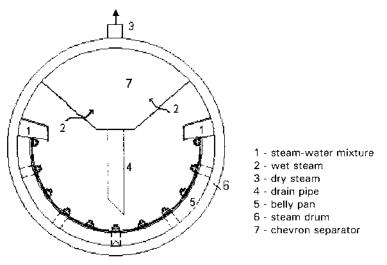
FIGURE 3.26 Arrangement of steam drum internals.
