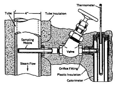
FIGURE 5.1 Throttling calorimeter.
