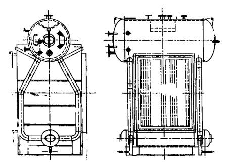
FIGURE 8.3 Boiler evaporator bundle.
