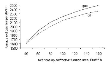
FIGURE 3.12 Furnace outlet temperature for gas and oil firing.
