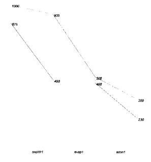
FIGURE 1.16a Performance of a HRSG with process steam use.
