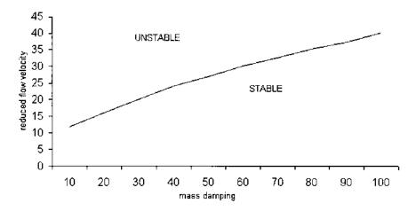
FIGURE 8.26 Damping factor versus nondimensional flow velocity.
