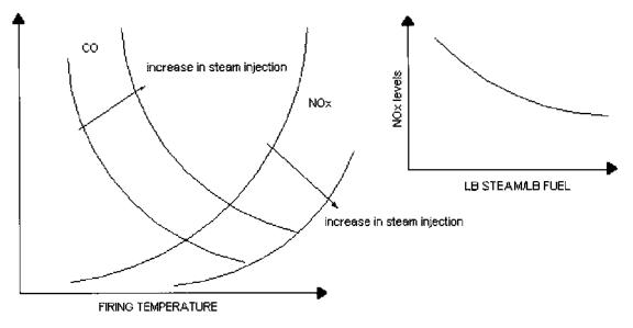
FIGURE 4.11 Effect of steam-water injection on NOx and CO.
