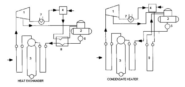
**FIGURE 1.18a** Secondary surfaces to improve HRSG efficiency. 1, turbine; 2, deaerator; 3, HRSG; 4, mixing tank; 5, pump; 6, deaerator coil; 7, condenser; 8, heat exchange; 9, condensate heater.
