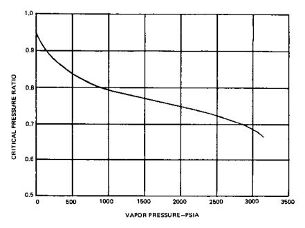
FIGURE 7.3 Critical pressure ratios for water.
