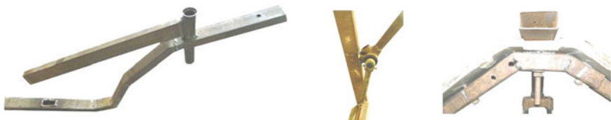
Fig. 8 Head frame with chassis rod (left), Integrated propulsion joint (middle), front head frame of the FRP hull (right)
