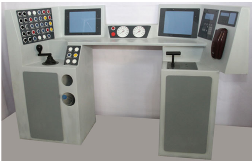
Fig. 9 Denotes the overall layout of the ideal workstation which is under evaluation of the motormen for freezing the design
