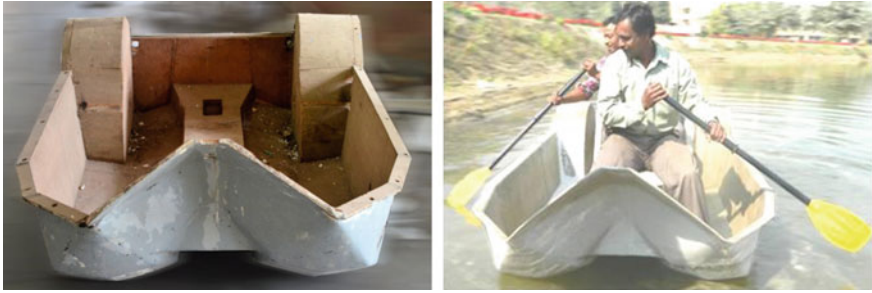
Fig. 9 View of catamaran type hull (left) and hull water testing (right)
