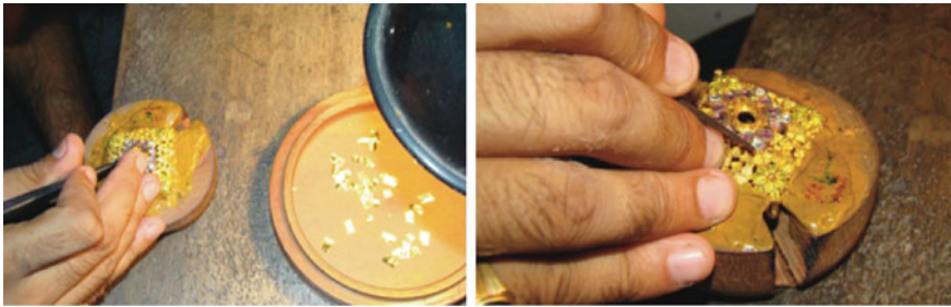
Fig. 3 Kundan setting process using very thin gold foils
