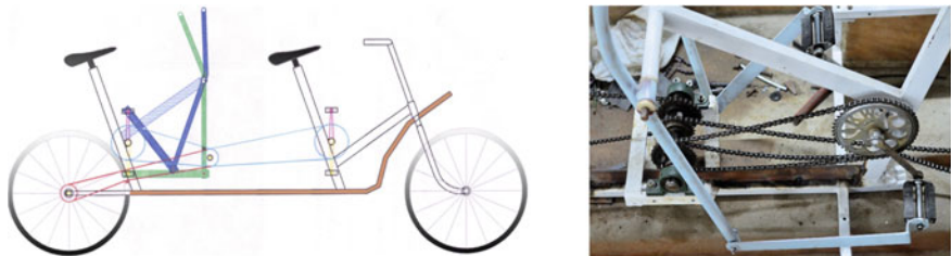
Fig. 7 CAD modeling of integrated mainframe (left) and cross trainer mechanized transmission system (right) of the ambulance
