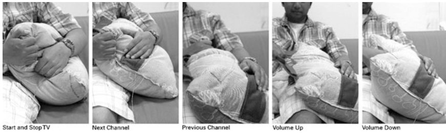
Fig. 7 Gesture sets for cushion remote (In order from left to right : starting and stopping TV, next channel, previous channel, volume up and volume down)
