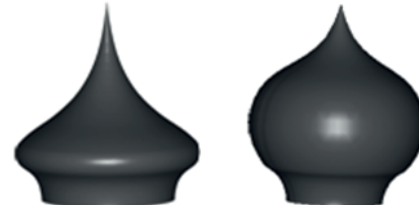
Fig.6. the streamline surface generated by changing the integration interval
