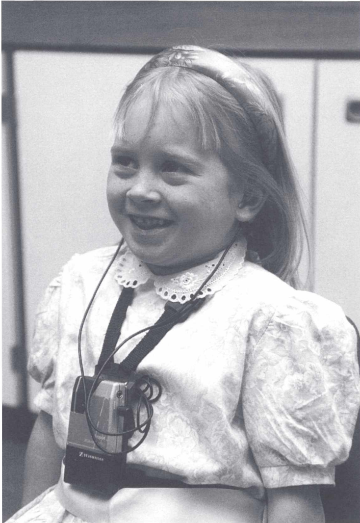
Figure 9.10. A Type II radio aid system in which the signal is passed from the body-worn radio receiver to the child's hearing aid via a lead.
