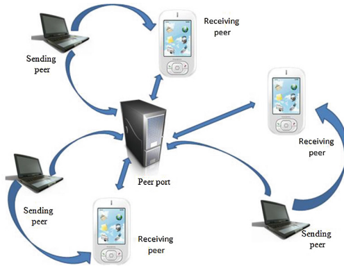
Fig. 4. Peer port is processing more than one request.
