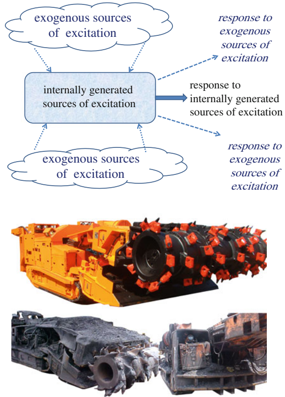
Fig. 2 Dynamic system depiction and pictures (courtesy of Joyglobal) of continuous mining machine
