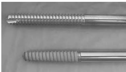
Figure 5 Bicylindrical uncoated 6 mm half-pin ( top ) is shown adjacent to a 5/6 mm tapered hydroxyapatite coated pin ( bottom ).
