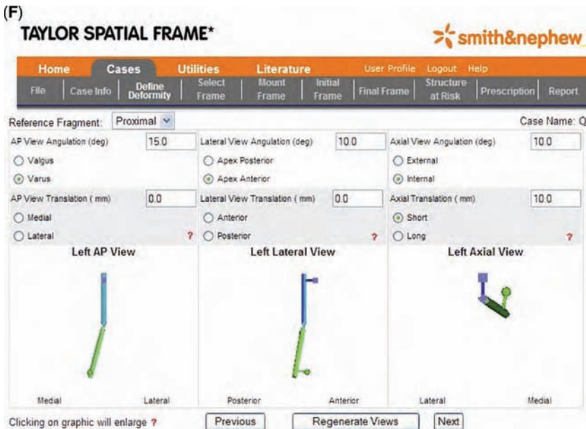
Figure 23.1 Case example of 37-year-old male with medial compartment arthritis after a medial plateau fracture. (F) The deformity data is entered into the web-based computer program and an image is generated recreating the deformity. (With reference to the stick diagrams, the blue box represents the knees and the green circle the foot.) (See p. 316)
