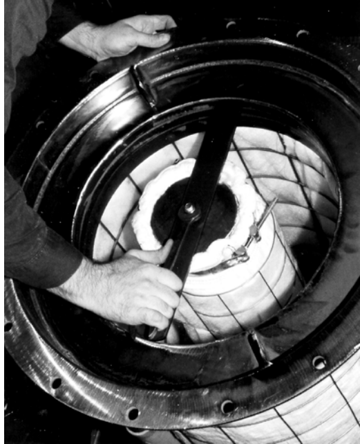
Figure 8.2 Filter within a filter (Monsanto Enviro-Chem Systems, Inc.).
