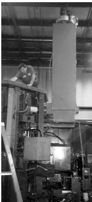
Figure 8.6 1000 ACFM on five-station machining center (Advanced Environmental Systems, Inc.).
