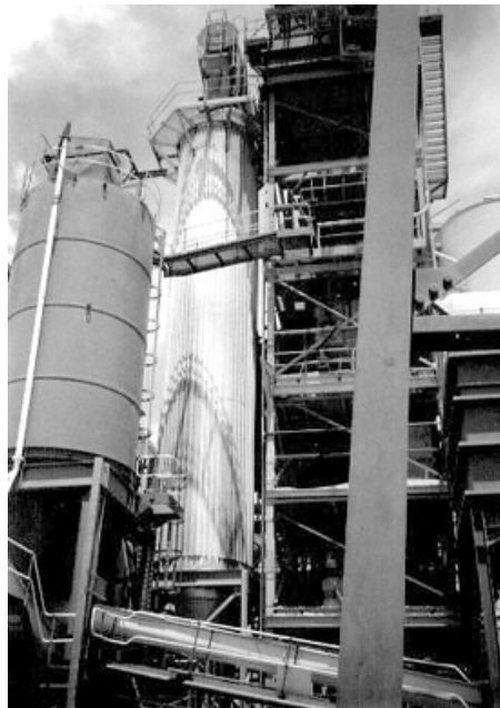
Figure 6.9 Evaporative cooler on dry process cement kiln (Hart Environmental, Inc.).
