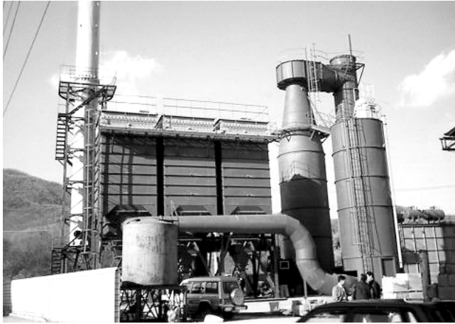
Figure 6.1 Evaporative cooler on pulse type baghouse (Bundy Environmental Technology).
