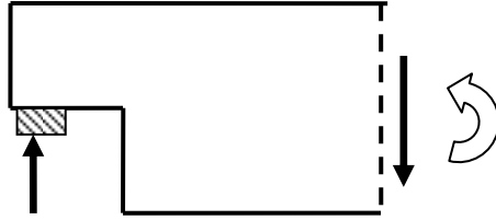
Fig. 18.9(a) D regions at a 'half' joint.
