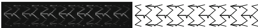
Fig. 6. Xience stent by Abbott (left); Computationally generated Xience-like stent (right) showing half of the mesh with n_C = 6 and n_L = 24 .
