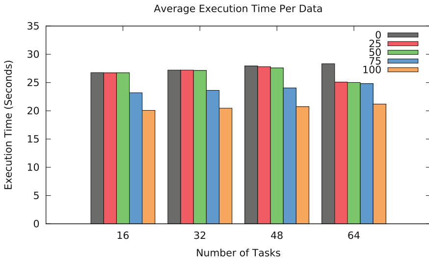
Fig. 12. This graph displays the results of our experiments as we increase the number of tasks per worker and as we incrementally perform upgrades to subsets of the cluster. The data here is normalized based upon data size, with the average execution time of data per configuration presented on the Y-axis. On the X-axis is the number of tasks assigned for the job in our 16 node cluster configuration.
