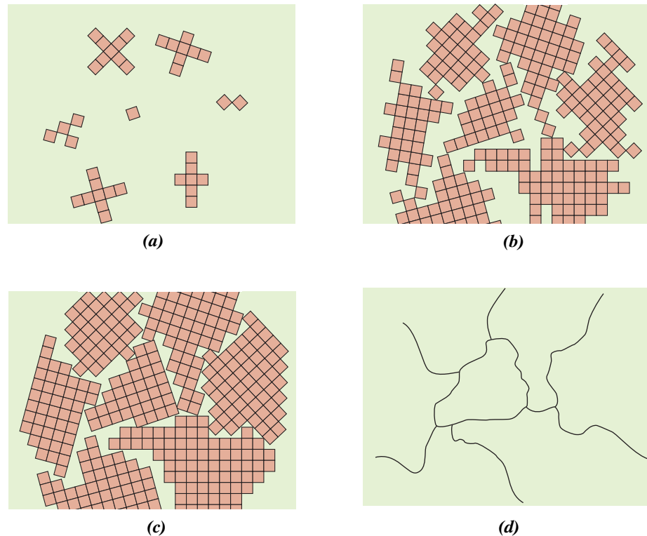
Figure 3.35 Schematic diagrams of the various stages in the solidification of a polycrystalline material; the square grids depict unit cells. (a) Small crystallite nuclei. (b) Growth of the crystallites; the obstruction of some grains that are adjacent to one another is also shown. (c) Upon completion of solidification, grains having irregular shapes have formed. (d) The grain structure as it would appear under the microscope; dark lines are the grain boundaries. (Adapted from W. Rosenhain, An Introduction to the Study of Physical Metallurgy , 2nd edition, Constable & Company Ltd., London, 1915.)
