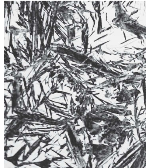
Figure 11.22 Photomicrograph showing the martensitic microstructure. The needle-shaped grains are the martensite phase, and the white regions are austenite that failed to transform during the rapid quench. 1220×. (Photomicrograph courtesy of United States Steel Corporation.)
