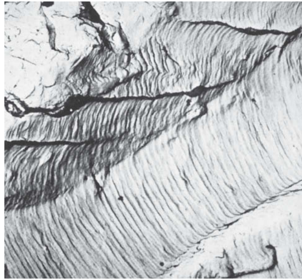
Figure 9.31 Transmission electron fractograph showing fatigue striations in aluminum. 9000 \times .
