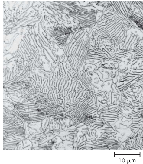
Figure 11.20 A photomicrograph of a pearlitic steel that has partially transformed to spheroidite. 1000 \times . (Courtesy of United States Steel Corporation.)
