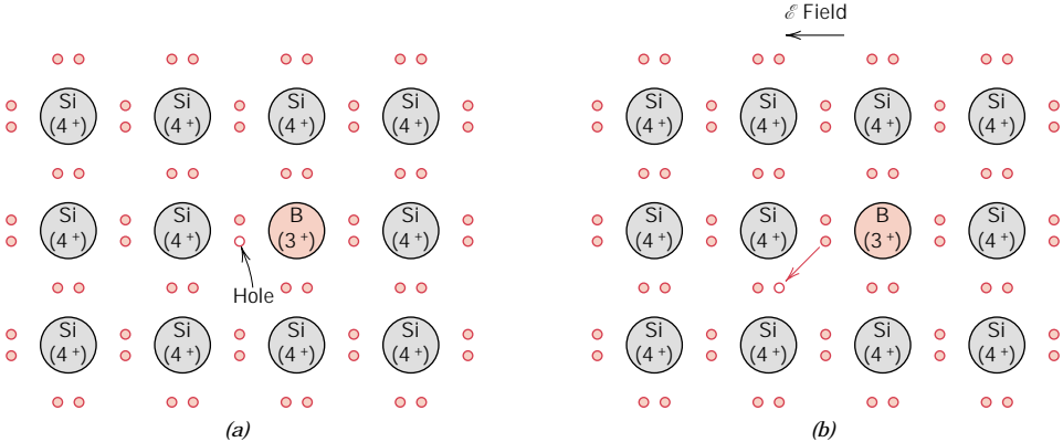
FIGURE 12.13 Extrinsic p -type semiconduction model (electron bonding). (a) An impurity atom such as boron, having three valence electrons, may substitute for a silicon atom. This results in a deficiency of one valence electron, or a hole associated with the impurity atom. (b) The motion of this hole in response to an electric field.
