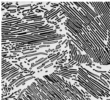
FIGURE 10.29 Photomicrograph of a eutectoid steel showing the pearlite microstructure consisting of alternating layers of \alpha ferrite (the light phase) and \text{Fe}_3\text{C} (thin layers most of which appear dark). 500 \times . (Reproduced with permission from Metals Handbook , Vol. 9, 9th edition, Metallography and Microstructures , American Society for Metals, Materials Park, OH, 1985.)
