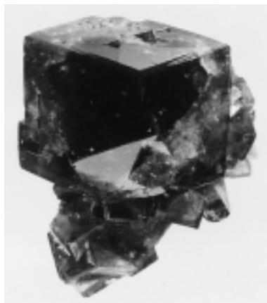
FIGURE 3.32 Photograph showing several single crystals of fluorite, \text{CaF}_2 . (Smithsonian Institution photograph number 38181P.)
