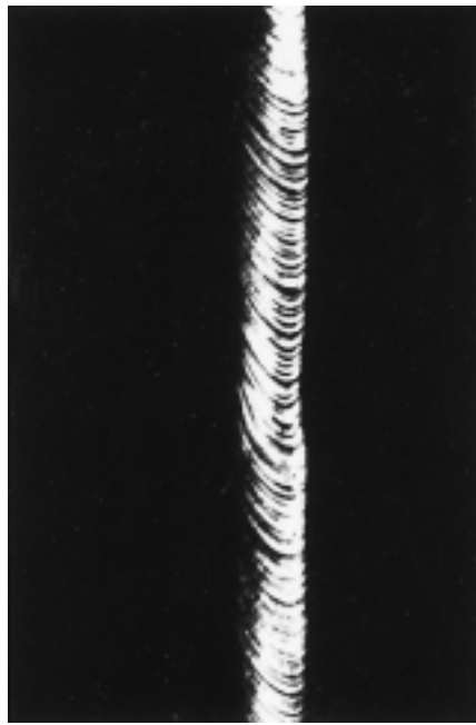
FIGURE 8.9 Slip in a zinc single crystal. (From C. F. Elam, The Distortion of Metal Crystals , Oxford University Press, London, 1935.)
