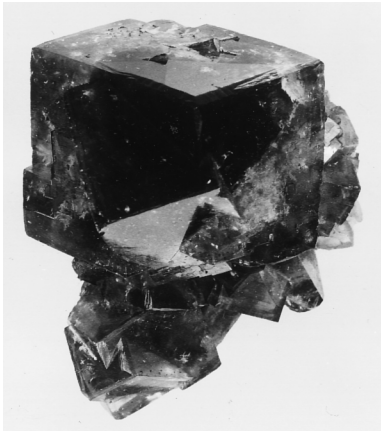
FIGURE 3.32 Photograph showing several single crystals of fluorite, \text{CaF}_2 . (Smithsonian Institution photograph number 38181P.)
