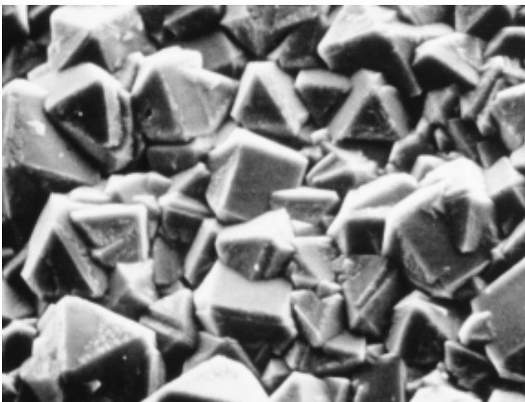
FIGURE 13.8 Scanning electron micrograph of a diamond thin film in which is shown numerous multifaceted microcrystals. 1000 \times . (Photograph courtesy of the Norton Company.)
