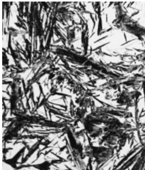
FIGURE 11.13 Photomicrograph showing the martensitic microstructure. The needle-shaped grains are the martensite phase, and the white regions are austenite that failed to transform during the rapid quench. 1220 \times . (Photomicrograph courtesy of United States Steel Corporation.)
