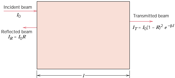
FIGURE 19.7 The transmission of light through a transparent medium for which there is reflection at front and back faces, as well as absorption within the medium. (Adapted from R. M. Rose, L. A. Shepard, and J. Wulff, The Structure and Properties of Materials , Vol. 4, Electronic Properties . Copyright © 1966 by John Wiley & Sons, New York. Reprinted by permission of John Wiley & Sons, Inc.)
