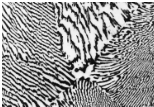
FIGURE 10.12 Photomicrograph showing the microstructure of a lead-tin alloy of eutectic composition. This microstructure consists of alternating layers of a lead-rich \alpha -phase solid solution (dark layers), and a tin-rich \beta -phase solid solution (light layers). 375\times . (Reproduced with permission from Metals Handbook , Vol. 9, 9th edition, Metallography and Microstructures , American Society for Metals, Materials Park, OH, 1985.)
