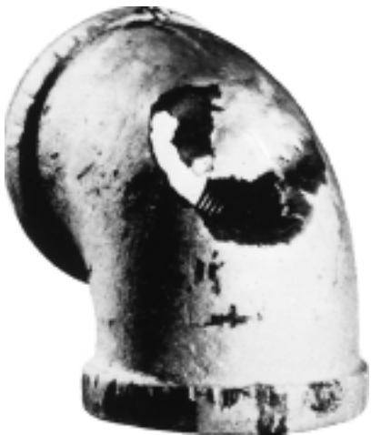
FIGURE 16.20 Impingement failure of an elbow that was part of a steam condensate line. (Photograph courtesy of Mars G. Fontana. From M. G. Fontana, Corrosion Engineering , 3rd edition. Copyright © 1986 by McGraw-Hill Book Company. Reproduced with permission.)
