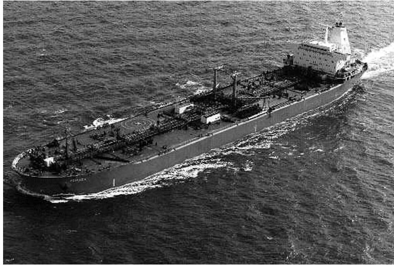
FIGURE 6-5 The “midsize” oil tanker Ventiza , built in 1986. It is 247 m (811 ft, or 2.7 U.S. football fields) long and 41.6 m (136 ft) wide. In 2000 the largest tanker in the world was the Jahre Viking , which is 458 m (1504 ft, or 5 U.S. football fields) long and 69 m (226 ft, or 0.89 U.S. football field) wide. From http://www.rigos.com/ventiza.html . Also see color insert.
