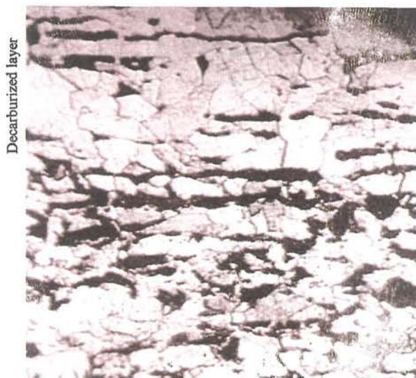
**Figure 8.15.** Microstructure of thermally decarburized steel.
