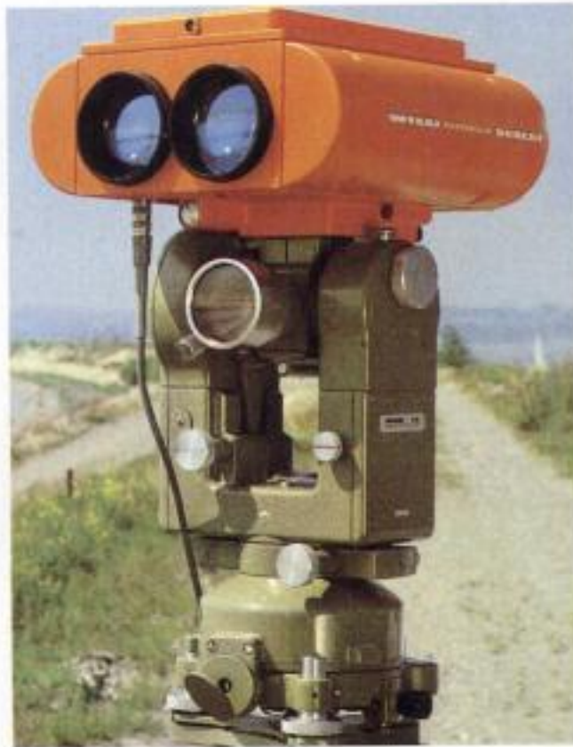
Fig. 11.2 EDM instrument Distomat DI 20 mounted on a theodolite (Courtesy : Leica AG, Switzerland)
