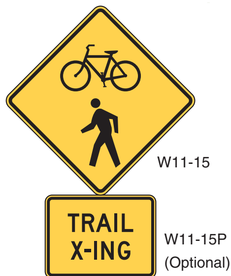
Figure 5-24. Advance Warning Assembly Example
