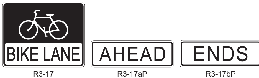
Figure 4-19. Bike Lane Sign
