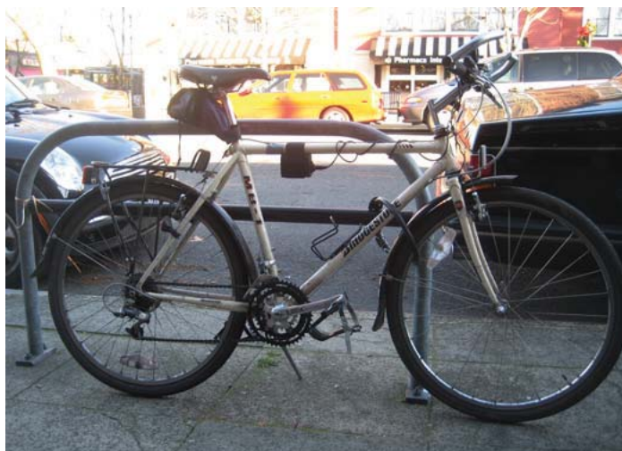
Figure 6-2. Example of “Inverted U” Bicycle Rack (Photo courtesy of Peter Lagerwey of Toole Design Group.)
