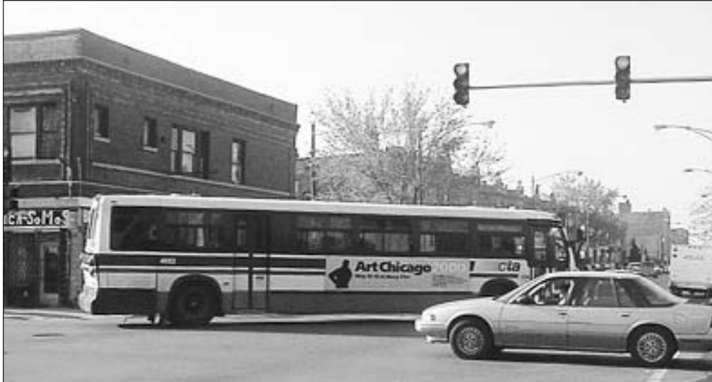
FIGURE 1-4 Transit Bus May Be Appropriate Design Vehicle for Urban Intersection Design
