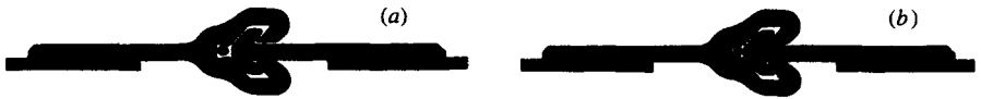
Figure 10-27 Water stop detail of Geolock screen. (a) Expansion profile before installation. (b) Final volume approximately after 40 hr. (BACHY.)
