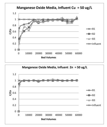
Figure 5. FBR breakthrough profiles for Cu(top) and Zn (bottom) from a synthetic stormwater solution onto granular manganese oxide (columns B1-B3 in series).
