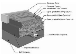
Figure 6. PICP with a no infiltration design using an impermeable liner
