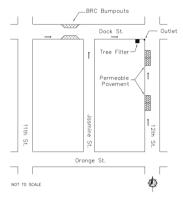
Figure 2: Layout of LID SCMs with arrows indicating direction of flow (not to scale)
