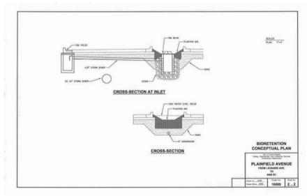
Figure 3: Section View - Bioretention Conceptual Plan
