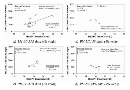
Figure 5. Relationship of Binder Data to APA Rutting Performance
