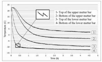
Figure 3. Data collected by the GLC for a system set to reach -20 °C as quickly as possible.
