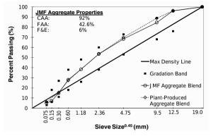
**Figure 1. Aggregate Properties**
