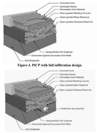
Figure 5.PICP with a partial infiltration design using an underdrain.
