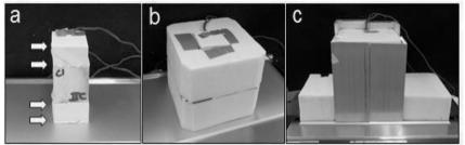
Figure 1. The guarded longitudinal calorimeter. a) The sample stack; b) the "stack-and-donut", instrumented and insulated; c) the complete GLC.
