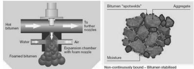
Figure 1 Foamed stablized based process illustration and final product (Figure from Whirgen)
