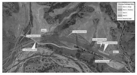
Figure 1 – Overview of New Project Drainage Area and LID Features
