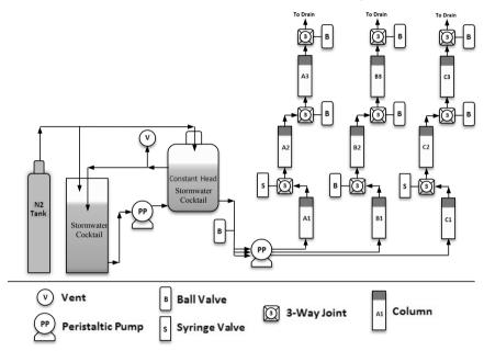
Figure 3. Experimental column setup (not to scale)
