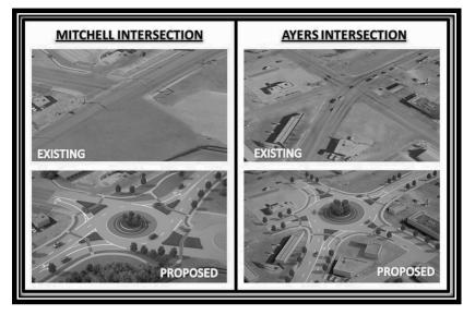
Figure 4 - Existing Conditions and Proposed Roundabouts at the Mitchell and Ayers Intersections.
