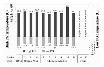
Figure 2. All Original Binder Continuous PG Data
