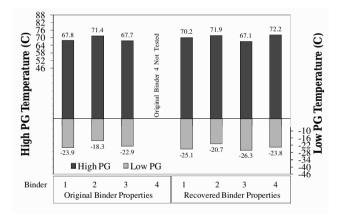
Figure 3. Original and Recovered Binder Continuous PG Data
