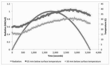
Figure 4. Data collected from the Solar Simulator for a hot mix asphalt sample.
