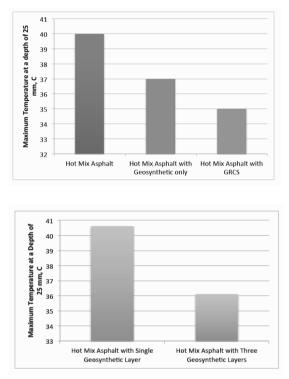
Figure 8. Results of experiments showing effect of chip seal and geosynthetic layer and thickness of geosynthetic layers
