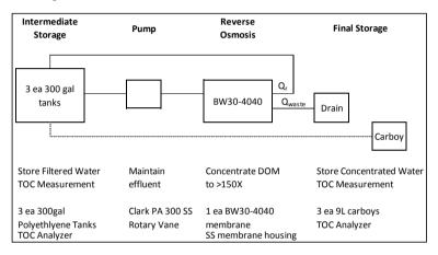
Figure 2. Schematic view of the concentration process using one Filmtech BW30-4040 membranes.
