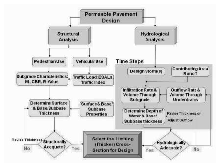
Figure 7. Permeable pavement design flow chart (Smith 2011)
