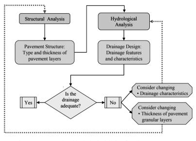
Figure 2. Structural and hydrological design flowchart [Swan 2009].
