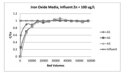
Figure 4. FBR breakthrough profiles for Cu(top) and Zn (bottom) from a synthetic stormwater solution onto granular iron hydroxide (columns A1-A3 in series).
