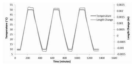
(b) Typical response of a concrete cylinder subjected to three heating and cooling cycles.
