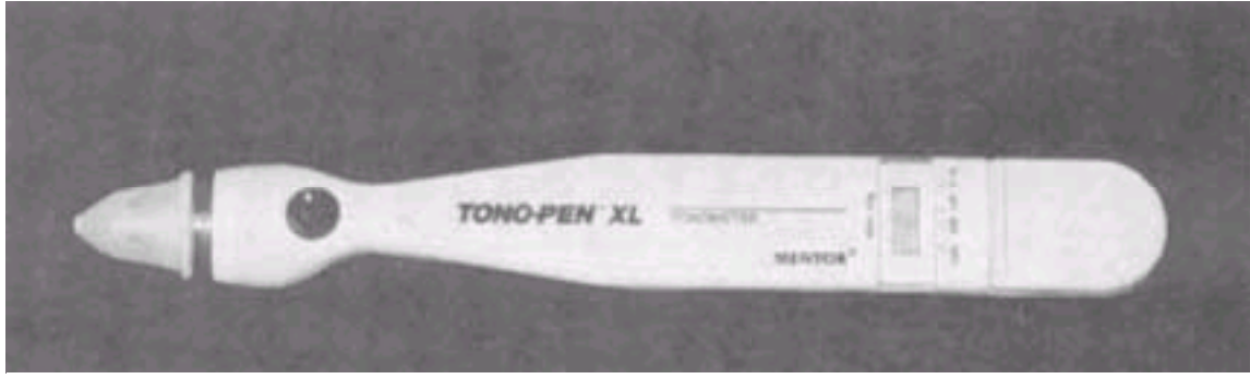
Figure 64-39 Bedside tonometry is easily accomplished with the Tono-Pen XL. The battery-powered device averages four consecutive readings and reports statistical reliability.
