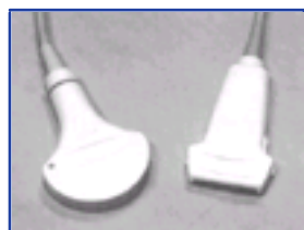
Figure 69-2 The curvilinear array probe is used for lower frequency (2.0 to 5.0 MHz) scanning of the abdomen and chest. It is best used for cardiac and abdominal imaging. The linear array probe is used for high frequency (6 to 10 MHz) scanning of superficial tissues, vessels, subcutaneous masses, and foreign bodies.
