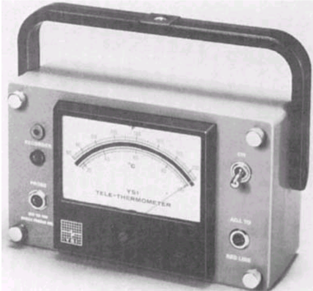
Figure 67-1 Electric thermometer (without probe). This is model 43TA with Fahrenheit and Celsius scales. Infrared tympanic membrane thermometers are acceptable alternatives, but the rectal probe has the advantage of providing a continuous readout. (Image courtesy of Yellow Springs Instrument Company, Yellow Springs, OH.)
