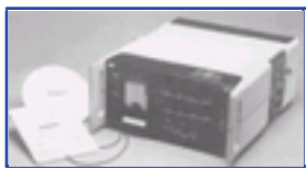
Figure 15-15 "Stand alone" transcutaneous pacemaker (Zoll NTP). This unit has a built-in monitor and strip chart recorder. (Courtesy of ZMI Corporation, Cambridge, Mass.)
