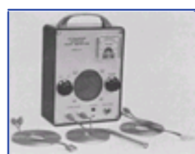
Figure 1-5 Ultrasonic Doppler flow detector with speaker and probes (model 811). (Courtesy of Parks Medical Electronics, Aloha, OR.)
