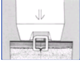
Figure 36-7 An anvil automatically bends the staple to the proper configuration. (From Edlich RF: A Manual for Wound Closure . St. Paul, MN, 3M Medical-Surgical Products, 1979. Reproduced by permission.)
