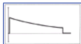
Figure 12-5 Monophasic truncated exponential waveform (MTE) (Energy delivered versus time/msec.) (Adapted courtesy of Cardiac Science, Inc., Irvine, CA.)
