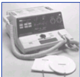
Figure 15-14 Combined defibrillator-transcutaneous pacemaker unit (Zoll-PD). The unit defibrillates through standard hand held paddles and has additional cable connections for electrocardiograph monitoring electrodes and for pacing electrodes. (Courtesy of ZMI Corporation, Cambridge, Mass.)
