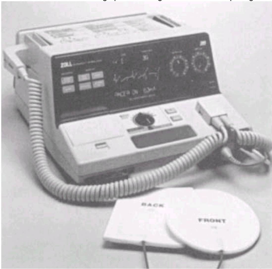
Figure 15-14 Combined defibrillator-transcutaneous pacemaker unit (Zoll-PD). The unit defibrillates through standard hand held paddles and has additional cable connections for electrocardiograph monitoring electrodes and for pacing electrodes. (Courtesy of ZMI Corporation, Cambridge, Mass.)
