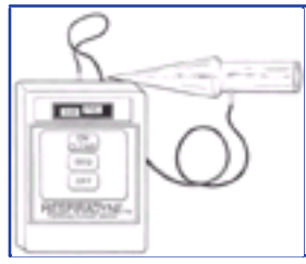
Figure 2-4 The Respiradyne portable spirometer. The device is turned on or "cleared" from the last effort. The patient exhales forcefully into the handheld mouthpiece following maximal inhalation. The "sequence" button permits selection of the desired spirometry measurements. The best of several tries should be recorded.
