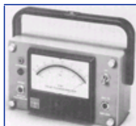
Figure 67-1 Electric thermometer (without probe). This is model 43TA with Fahrenheit and Celsius scales. Infrared tympanic membrane thermometers are acceptable alternatives, but the rectal probe has the advantage of providing a continuous readout. (Image courtesy of Yellow Springs Instrument Company, Yellow Springs, OH.)
