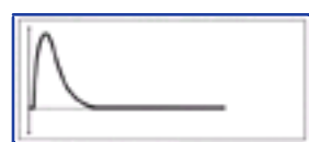
Figure 12-4 Monophasic damped sine waveform (MDS) (Energy delivered versus time/msec.) (Adapted courtesy of Cardiac Science, Inc., Irvine, CA.)
