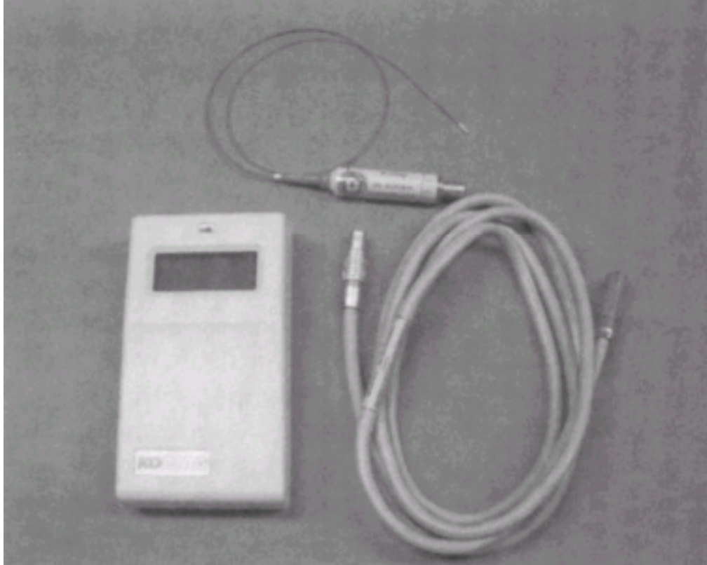
Figure 55-2 The HANDY electronic transducer-tipped catheter system (Courtesy of Mammendorfer Institute for Physics and Medicine LTD. Munich, Germany.)
