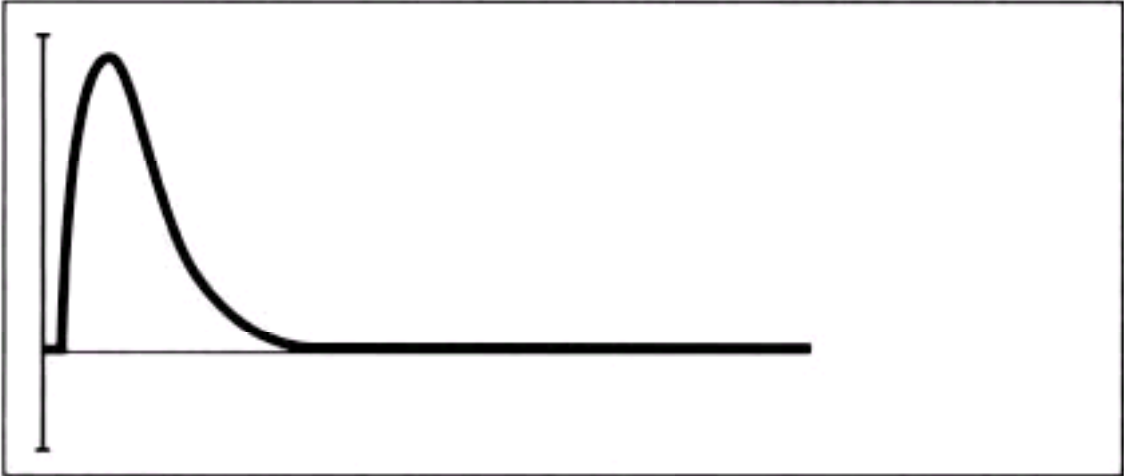
Figure 12-4 Monophasic damped sine waveform (MDS) (Energy delivered versus time/msec.) (Adapted courtesy of Cardiac Science, Inc., Irvine, CA.)
