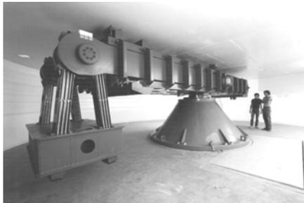
**FIG. 7: Geotechnical centrifuge at the University of Colorado at Boulder**
