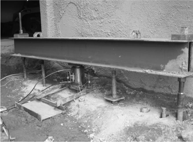
**FIG.5. Dial gauges for micropile test**
