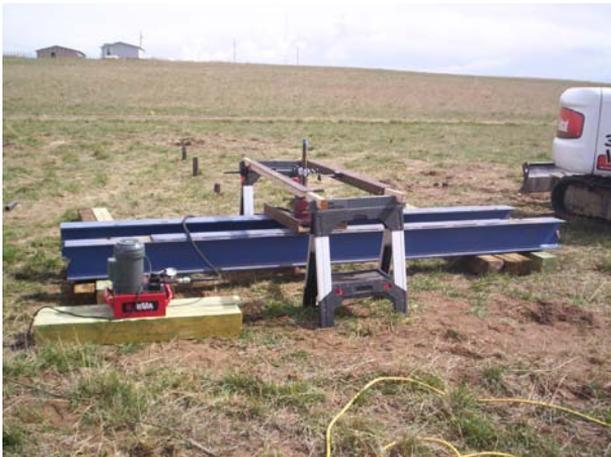
**FIG. 3. Typical Tension Test Load Frame Setup**
