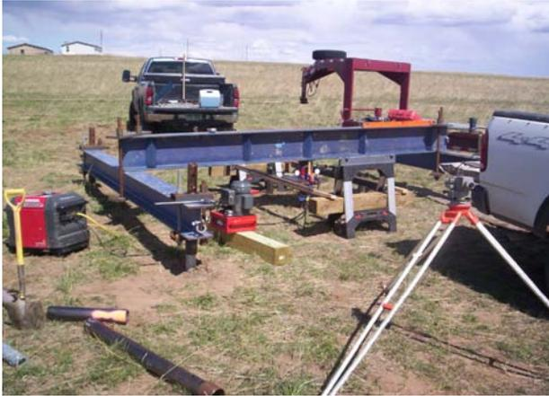
**FIG. 2. Typical Compression Test Load Frame Setup**
