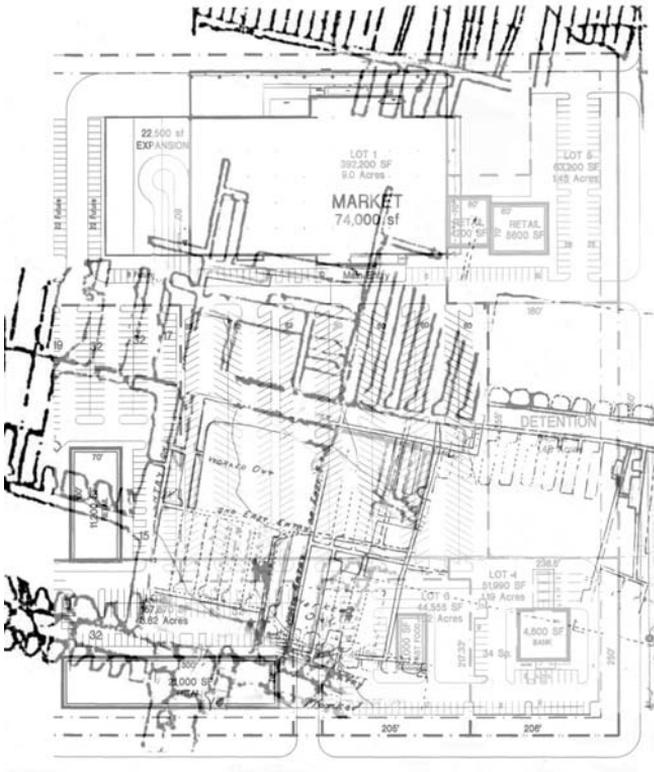
**FIG. 3. Mine map overlay on shopping center development plan.**
