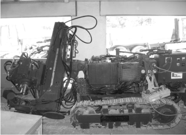
**FIG.2. Hydraulic drill rig**
