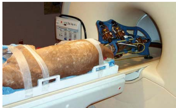
Fig. 28.9. The MR compatible robot (MrBot) developed for prostate brachytherapy at Johns Hopkins tested in an animal study
