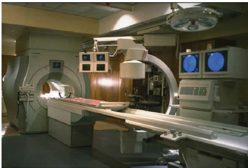
Fig. 8.4. Interventional MRI suite combining 1.5-T MRI and C-arm angiography systems. (Courtesy of Philips Medical Systems Ltd)
