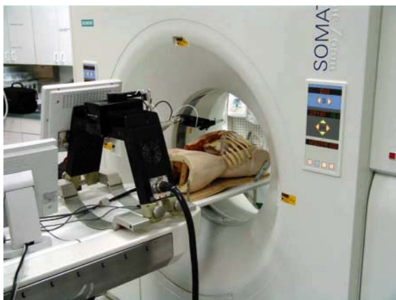
Fig. 28.6. The AcuBot robot system, used for needle placement in respiratory lung phantom during CT-fluoroscopy
