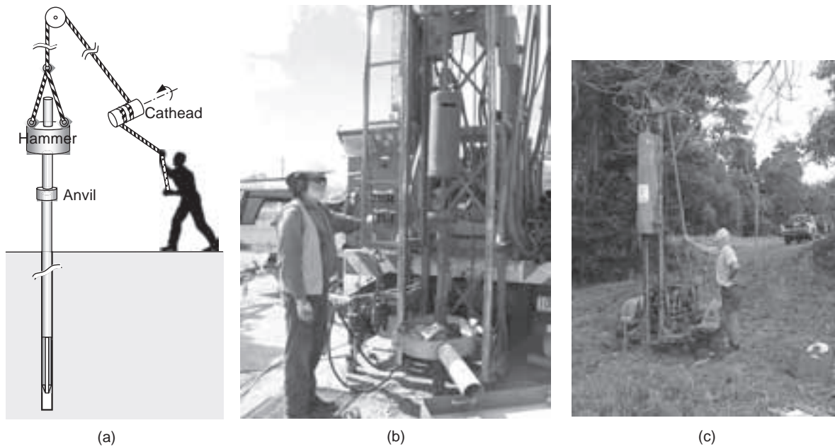
Figure 11.5 Penetration tests: (a) schematic diagram of SPT (b) photograph of SPT (Courtesy of Mr. Mark Arnold) (c) photograph of a dynamic cone penetration test rig
