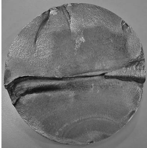
PHOTO 2.1 Fatigue failure of an agitator shaft.
