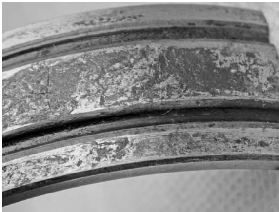
PHOTO 10.14 A heavily fretted surface with a visible crack.
