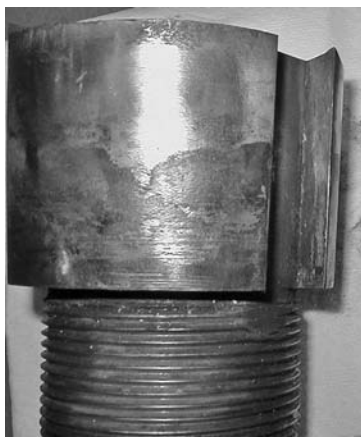
PHOTO 7.4 The ugly blackened area on this pump shaft is fretting caused by movement between the impeller and the shaft.
