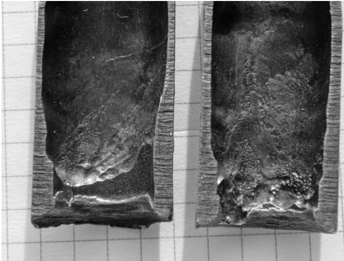
PHOTO 7.10 Erosion corrosion of two heat exchanger tubes.
