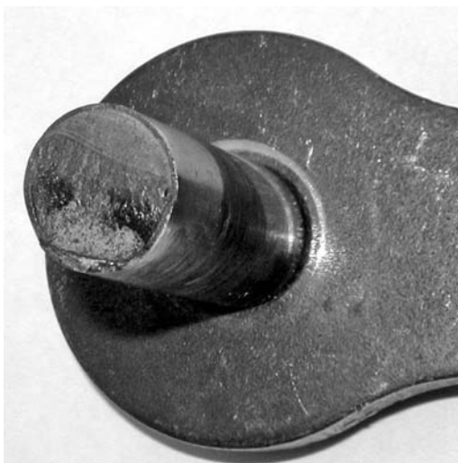
PHOTO 13.2 The fatigue fracture of a case-hardened pin.
