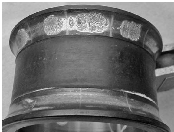
PHOTO 10.32 This ball path shows a combinatin of problems, probably brinelling combined with an inadequate lubricant.
