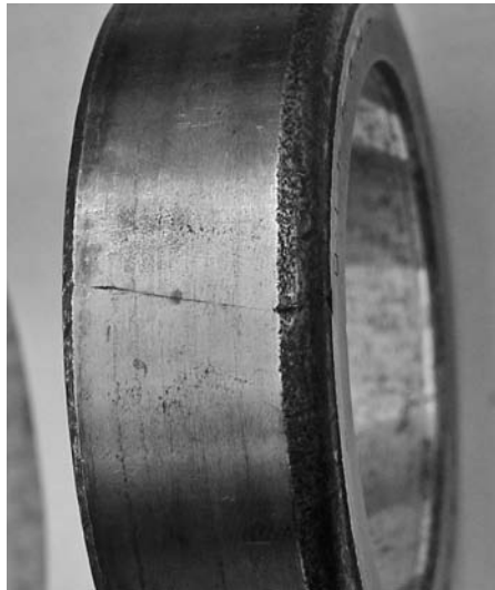
PHOTO 10.1 Note the crack in this surface-hardened race. It has not propagated through to the roller path.
