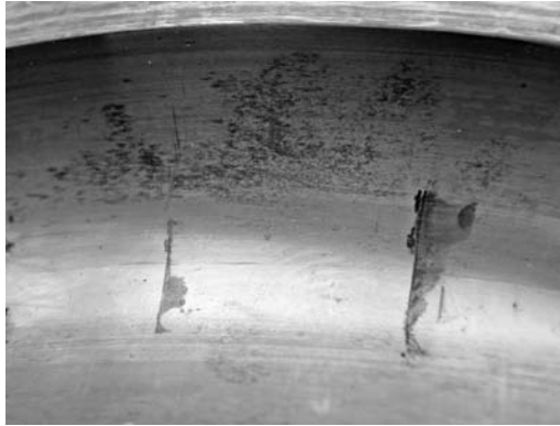
PHOTO 10.6 The two black lines are water spots (corrosion damage) on a ball path.
