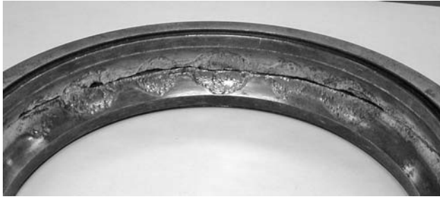
PHOTO 10.28 A brinelled bearing that ran for 9 months.
