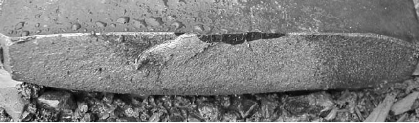
PHOTO 4.17 This brittle fracture of a left truck fork started at the old cracks (notches) in the center.
