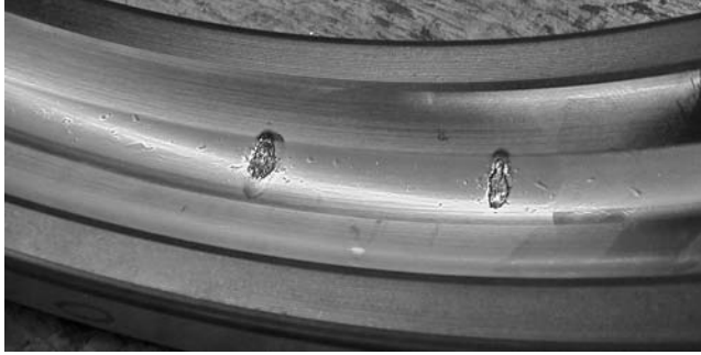
PHOTO 10.23 These two spalls are located on the ball centers.
