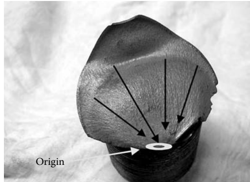
PHOTO 4.8 A reducer input shaft failure. We've put a series of lines on the surface to accent the "Chevron marks" that point to the crack origin.
