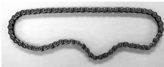
PHOTO 13.1 A chain wears every time the links flex. There are 10 wear points on this chain compared with four on a properly adjusted one.
