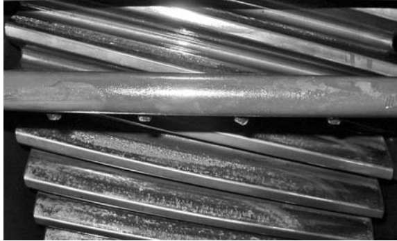
PHOTO 11.24 The varying pitting on these teeth show there are machining inconsistencies.
