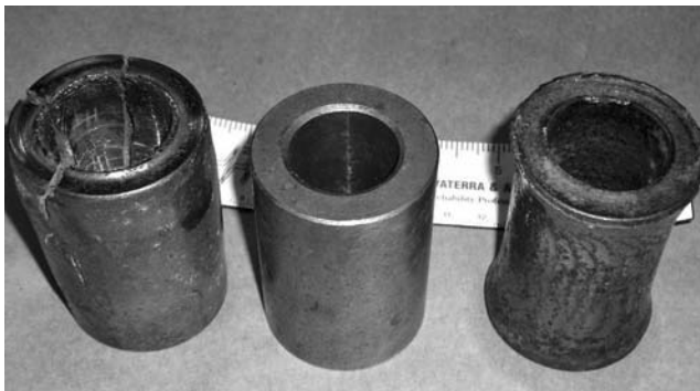
PHOTO 4.1 Three conveyor rollers. The center one is “as supplied,” while the outer two have failed from contact stresses. The left roller was case hardened and cracked, while the right roller was unhardened and ductily deformed.
