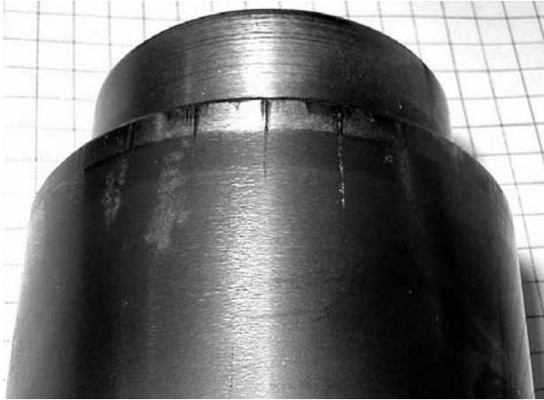
PHOTO 10.26 A forklift truck spindle that has been brinelled by careless assembly procedures.
