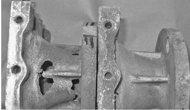
PHOTO 2.2 Pitting corrosion resulting from elevated temperatures on an aluminum housing.
