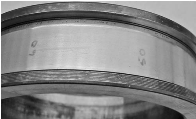
PHOTO 10.35 Mechanical fluting of a roller bearing from a steel mill drive.
