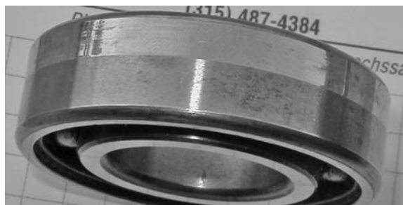
PHOTO 10.8 The design called for only \frac{1}{2} of this bearing to be supported — and the fit was very loose.
