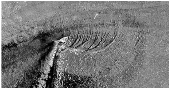
PHOTO 6.8 The river marks show the crack took a sudden left turn.
