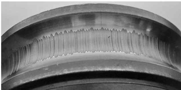
PHOTO 10.33 “Fluting” from electrical discharge in a variable speed motor.
