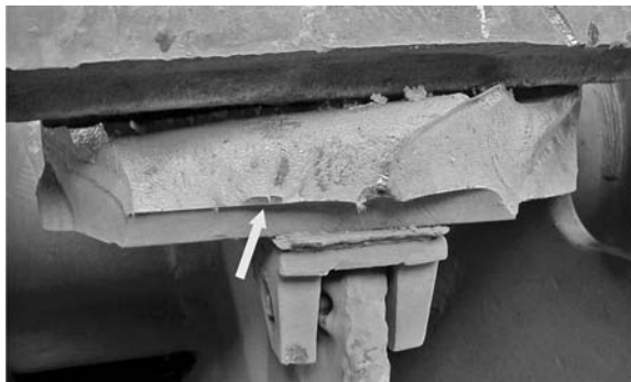
PHOTO 4.15 An overall view of the broken hammer. This brittle fracture started at the arrow.
