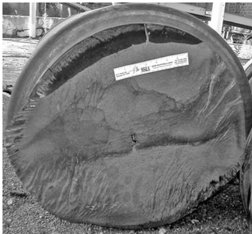
PHOTO 6.11 A roll from a steel mill. The blackened area is an older oxidized crack surface. The IZ is the lower third of the roll.
