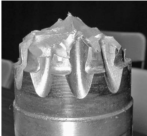
PHOTO 6.2 A torsional fatigue failure with multiple origins.
