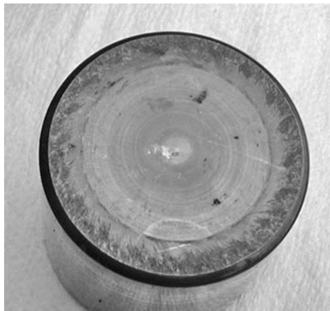
PHOTO 10.43 The “semi-colons” on the end of this roller testify that very high thrust loads have occurred.
