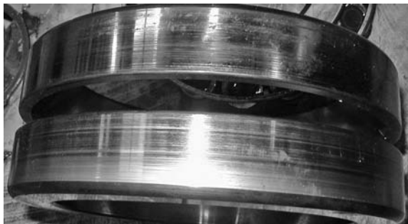
PHOTO 10.10 Both of these bearings were loose in the housing and the movement has polished the races.
