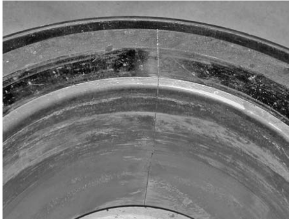
PHOTO 10.15 The cracked inner ring of a through-hardened bearing.
