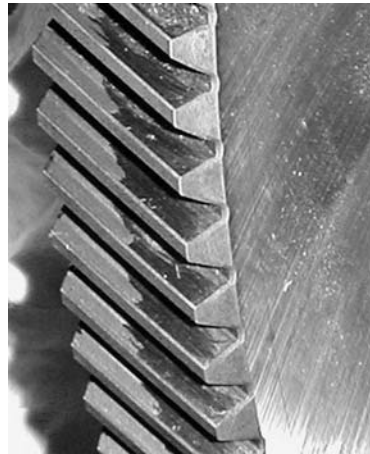
PHOTO 11.13 The harmless micropitting on these teeth show up as bands where the machining has left minute ridges.
