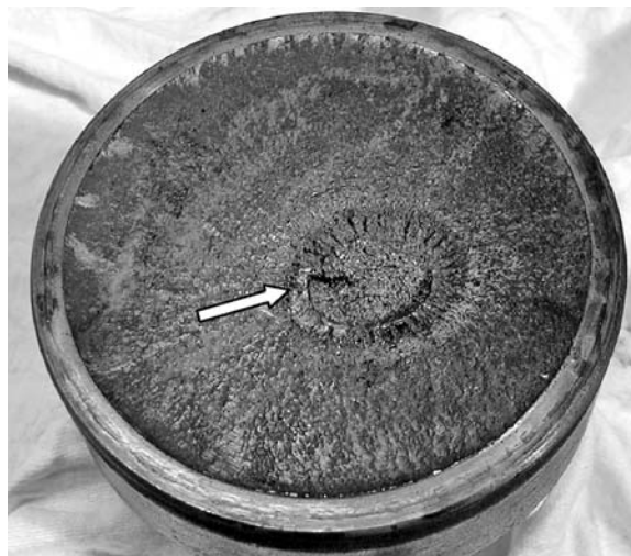
PHOTO 5.7 A rotating bending failure with multiple origins around the perimeter. The small IZ indicates the shaft was lightly loaded at the time of final failure.
