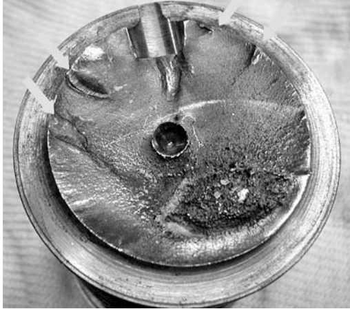
PHOTO 5.11 A rotating shaft that has failed. The keyway position, ratchet marks, and IZ shape all give clues to the failure cause.
