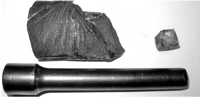
PHOTO 4.2 Torsional overload failures of a through hardened truck axle and an inexpensive socket wrench extension. Note the difference in appearance.
