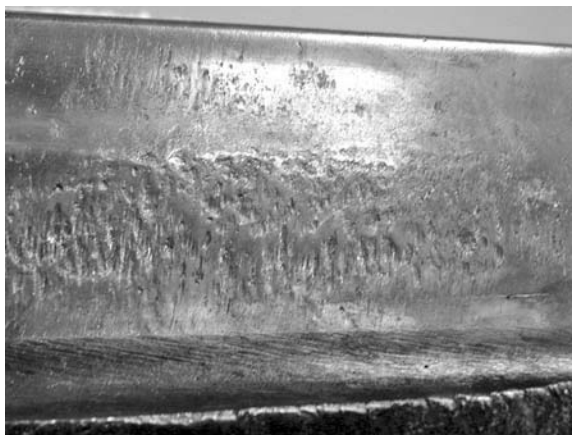
PHOTO 8.1 Adhesive wear of a through-hardened gear tooth.
