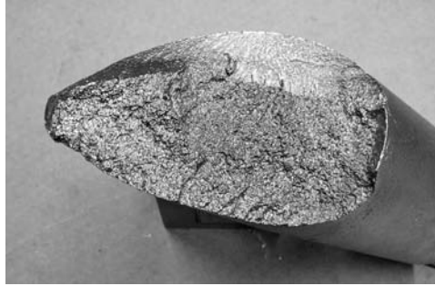
PHOTO 6.1 A classic torsional fatigue with a single origin. The coarse, rough IZ is because this shaft is ductile iron.
