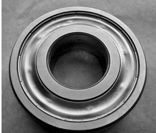
PHOTO 10.5 A motor bearing where an overzealous oiler with an electric grease gun collapsed the shield.
