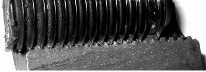
PHOTO 8.2 The bolt has welded itself to the steel flange.
