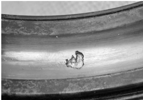
PHOTO 10.25 Another Hertzian fatigue spall.
