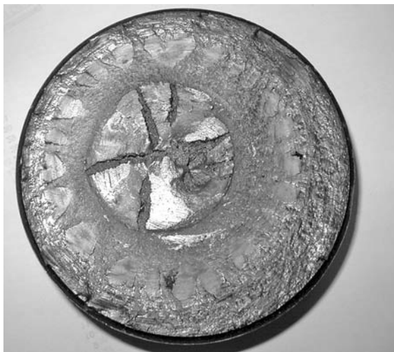
PHOTO 6.12 The very low cycle torsional fatigue failure of a large machine shaft.
