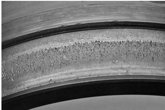
PHOTO 10.29 This “peeling” is frequently seen when the lubricant is inadequate.
