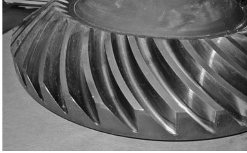
PHOTO 11.3 A spiral bevel gear — resulting in smoother power transmission than the bevel gear.
