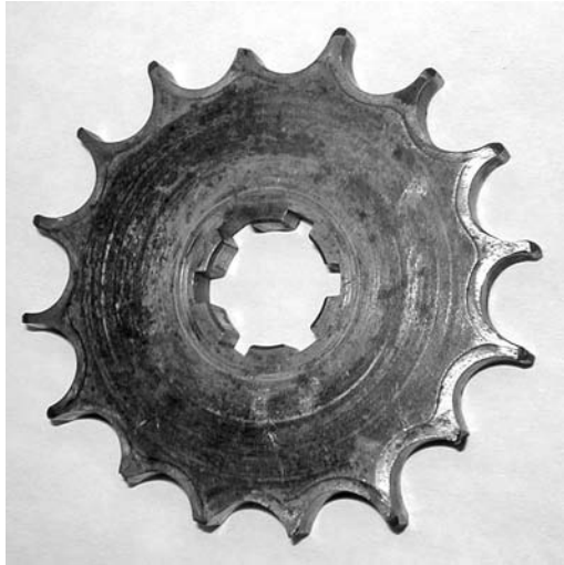
PHOTO 13.3 A born worn unhardened sprocket.
