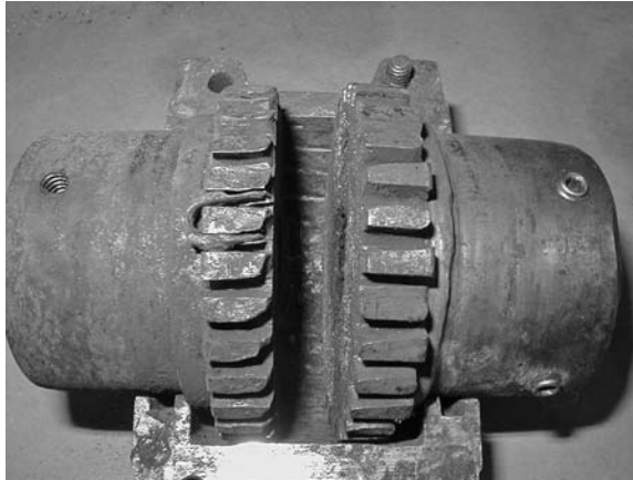
PHOTO 13.5 An improperly lubricated and badly aligned grid coupling.
