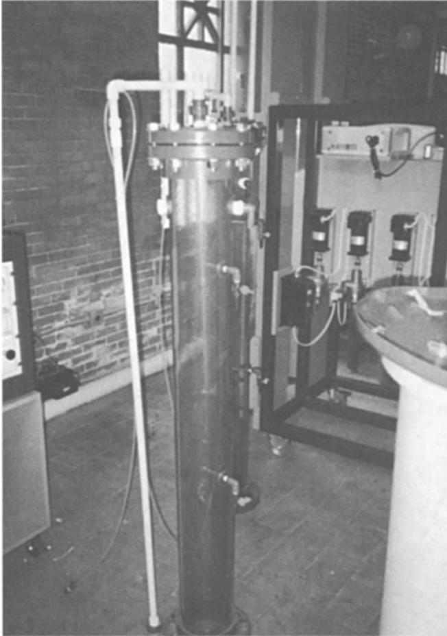
FIGURE 28.4 Top section of filter column preassembled with quick-connect unions, flanged sections bolted together. (Courtesy of CDM.)
