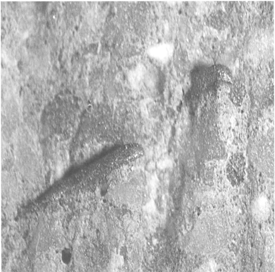
Figure 2.41 Shadow zones, formed behind reinforcement fibres during water jet erosion (Hu et al., 2004)
