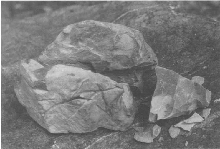
Figure 6.31 Rock sample crushed with the explosive pellet impingement technique (Becker et al., 1999)
