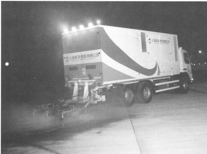
Figure 4.3 Unit for runway cleaning (photograph: WOMA Apparatebau GmbH, Duisburg)
