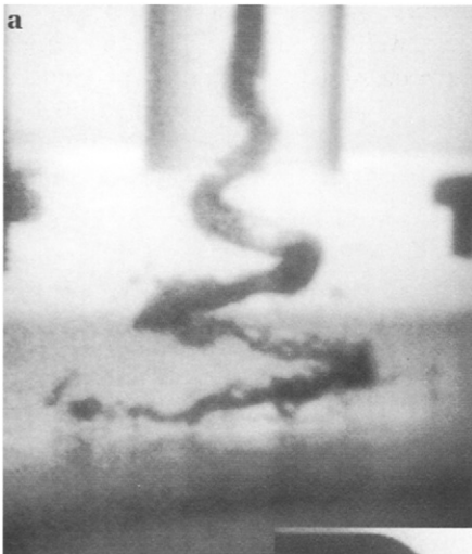
Figure 7.25 Appearance of self-resonating water jets; f_p=4.6 kHz (photograph: Dynaflo ® , Inc., Jessup) a - v_j=94.5 m/s; b - v_j=89.9 m/s; c - v_j=83.8 m/s
