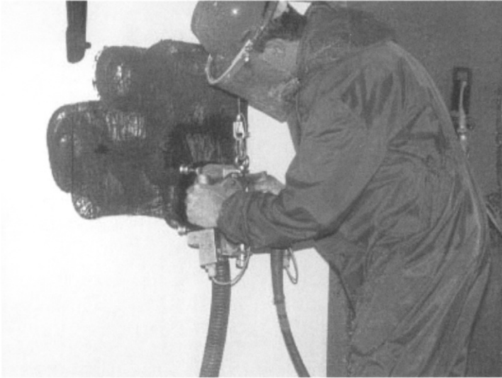
Figure 3.18 Emission-free performing hydroblasting tool (WOMA Apparatebau GmbH, Duisburg)
