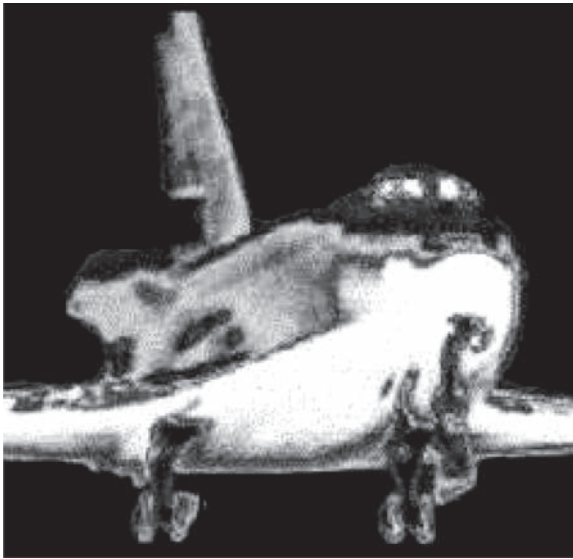
Figure 5.7 Thermographic image of a space shuttle in a hypersonic wind tunnel
