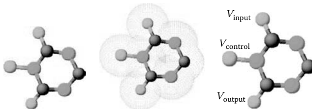
FIGURE 7.37 Three-terminal MF device comprised from a cyclic molecule with a carbon interconnecting framework.
