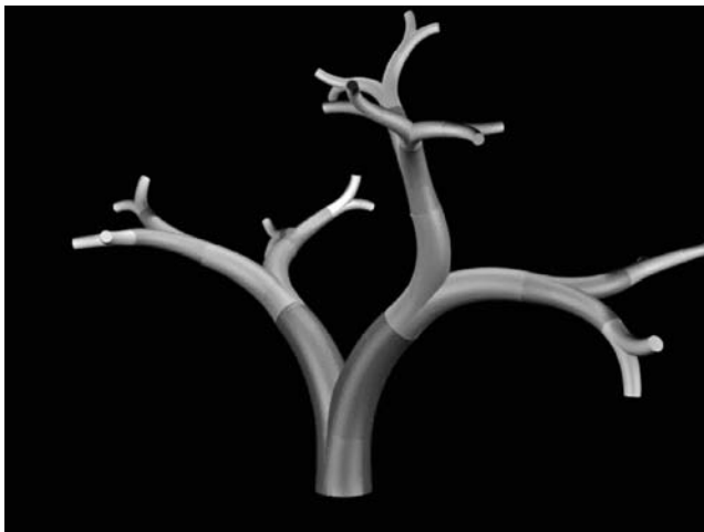
FIGURE 22.11 An illustration of a four-level dendritic neural tree made of 14 symmetric Y-junctions of the type in Figure 22.10. (From D. Srivastava, M. Menon, and K. Cho, Computing in Engineering and Sciences (CISE), an IEEE and APS publication, 42 (2001). With permission.)
