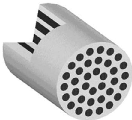
FIGURE 21.7 Typical bicomponent islands-in-the-sea fiber.
