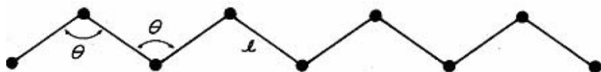
Figure 1.3. The fully extended all-trans configuration of a carbon-carbon chain (After Kaufman and Falcetta, 1977, copyright 1997 John Wiley & Sons, Inc. Reproduced with permission)
