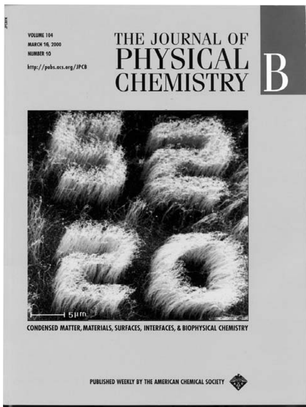
Figure 6.24. A typical SEM image of an aligned nanotube pattern prepared by the pyrolysis of FePc onto the photoresist prepatterned quartz via micromolding technique, appeared in a cover page of The Journal of Physical Chemistry (After Huang S. et al. , 2000, copyright 2000 The American Chemical Society. Reproduced with permission)
