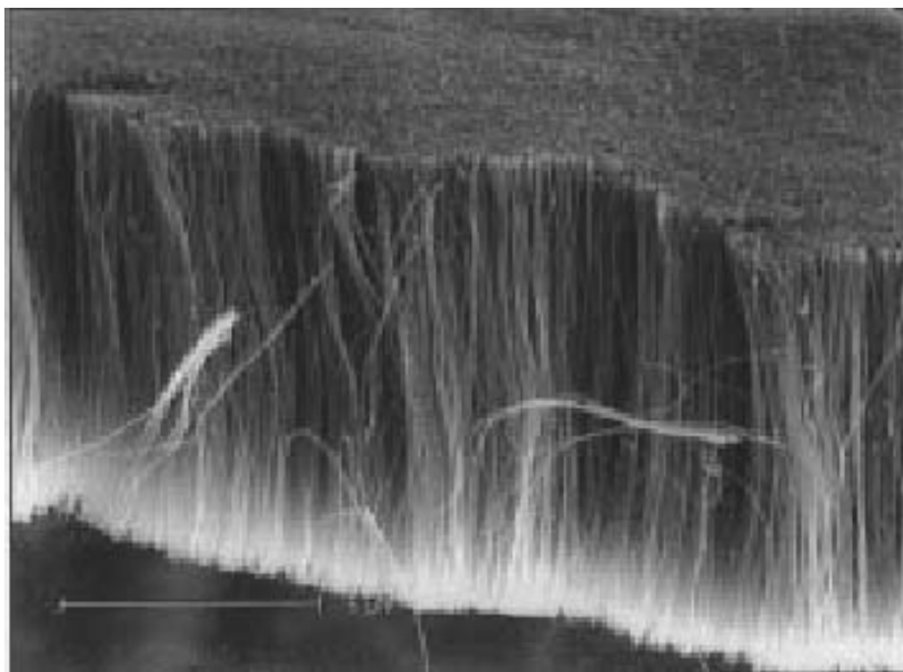
Figure 6.19. A typical SEM image of the aligned carbon nanotube film prepared by pyrolysis of FePc. The misalignment seen for some of the nanotubes at the edge was caused by the peeling action for the SEM sample preparation (After Huang S. et al. , 1999, copyright 1999 The American Chemical Society. Reproduced with permission)
