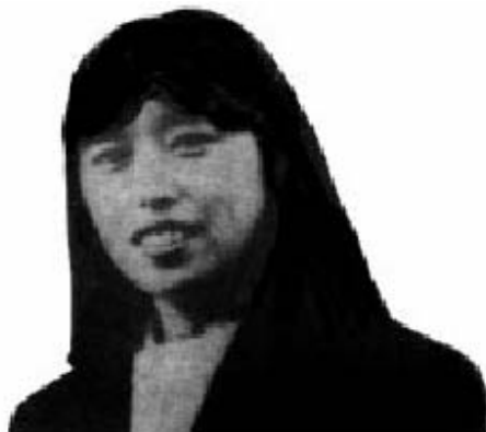
Figure 3.20. Light image formation on polyaniline-TiO 2 film immersed in 0.5 mol/l phosphate buffer (pH 7) containing 20 wt% methanol by projecting the positive image on the polyaniline-TiO 2 film with illumination by 500 W xenon lamp for 1 min (After Yoneyama et al. , 1992b, copyright 1992 The Royal Society of Chemistry. Reproduced with permission)
