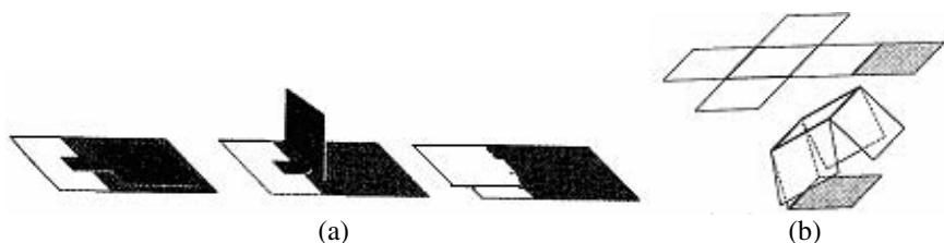
Figure 11.2. (a) The actuation paddles consist of rigid square plates with surface dimensions of 90 \mu\text{m} on bilayer hinges of 30 \mu\text{m} by 30 \mu\text{m} . From left to right: paddles lie flat at 0^\circ ; paddles are perpendicular to the surface around 90^\circ ; paddles lie flat at 180^\circ . The position of the paddles is controlled by the applied voltage; (b) schematic representation of actuators with three consecutive rigid elements forming the closed cubic box (After Smela et al. , 1995, copyright 1995 American Association for the Advancement of Science)
