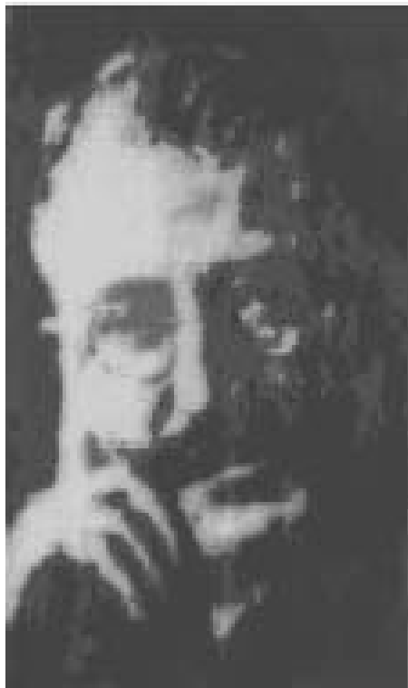
Figure 3.24. Photoluminescent pictures (excitation at 365 nm) of Hermann Staudinger produced by photobleaching an oriented EHO-OPPE/UHMW-PE blend film for 120 min, using a photomask that was fabricated by conventional laser printing of an image onto a transparency film (After Kocher et al. , 2001, copyright 2001 Wiley-VCH Verlag. Reproduced with permission)
