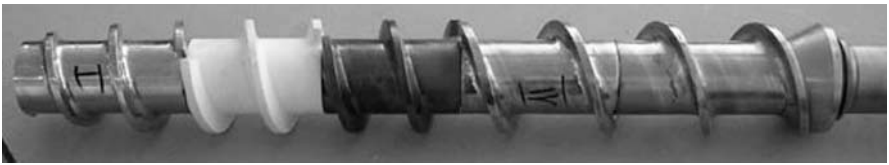
Fig. 10 Hybrid auger with metallic and ceramic segments ( \varnothing 80mm, L_{\text{auger}}=835 mm)
