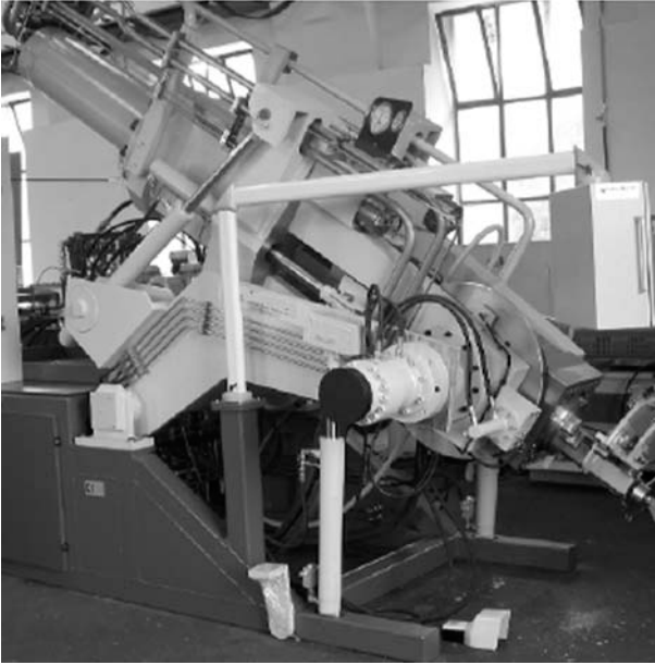
Fig. 12 Piston extruder for hard metal with automatic tool changing device
