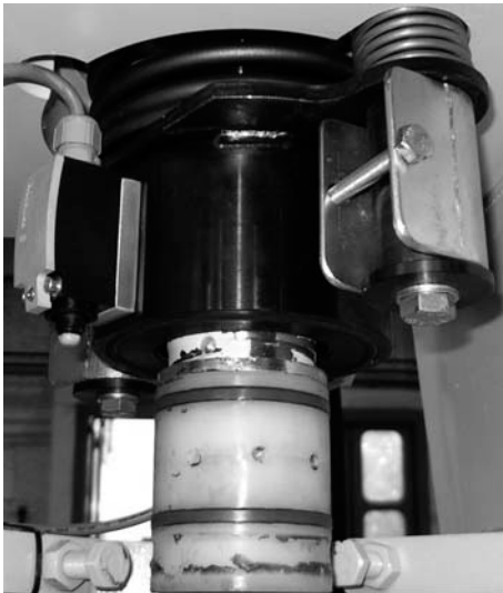
Fig. 10 Press ram in cleaning position
