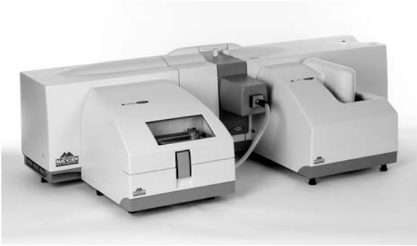
Fig. 5 Laser particle sizer (photo: Malvern)
