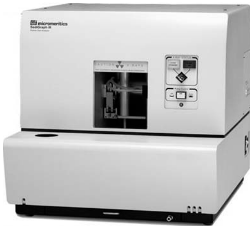
Fig. 4 Sedigraph 5100 for measuring the grain size distribution (photo: Micro-meritics)
