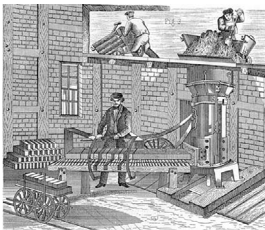
Fig. 16 First upright auger extruder powered by steam, 1858
