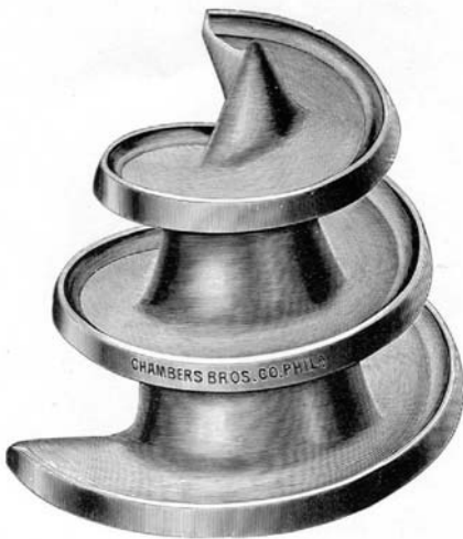
Fig. 31 Auger design of American extruders 1900/1920: expression screw for sandy or very loamy clay
