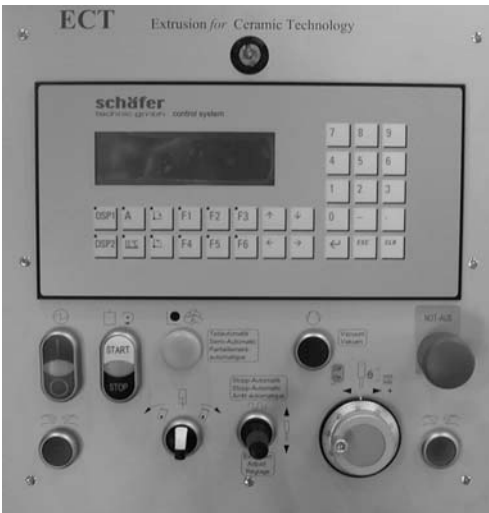
Fig. 7 Panel of a micro-processor based control system
