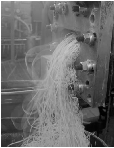
Fig. 21 Discharge of granulated catalyst carriers
