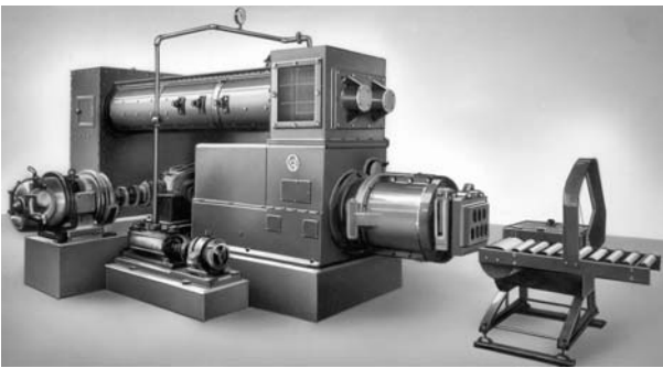
Fig. 47 Combined de-airing extrusion machine comprising of vacuum double-shaft mixer and auger extruder, 1937
