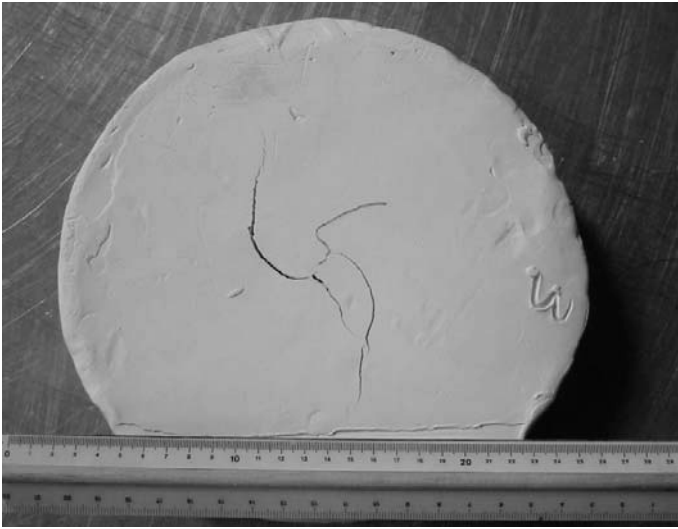
Fig. 10 Slug showing a Y-shaped drying crack resulting from a triple-blade point auger
