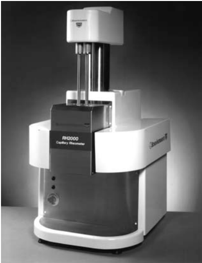
Fig. 9 Twin bore capillary rheometer (photo: Malvern)
