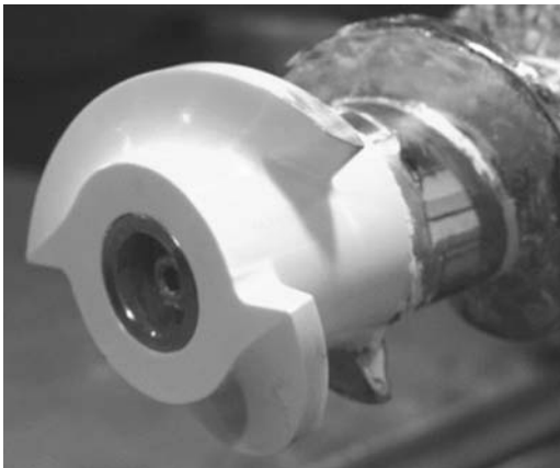
Fig. 6 Steel auger with ZrO_2 – front auger
