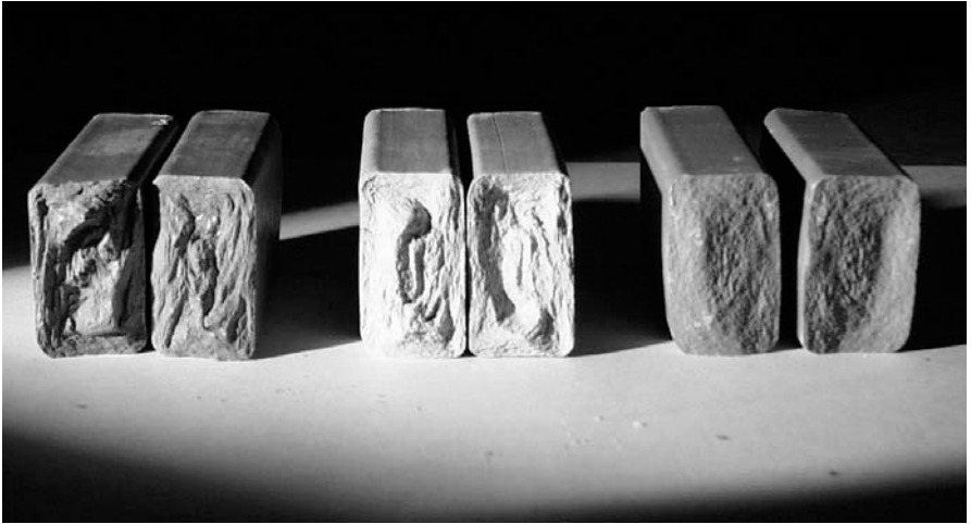
Fig. 3 Flow laminations in cross-section of clay-body columns Left: very plastic clay; Centre: kaolinitic kaoline; Right: clay with grog addition
