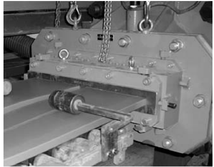
Fig. 17 Combination pressure head and die assembly for extruding roof-tile slugs; 2 side-by-side columns
