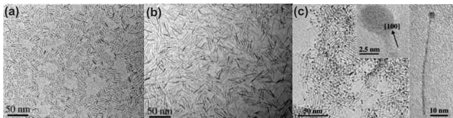
Fig. 3.4. a–c TEM overview images of titania nanorods with lengths of a 12 and b 30 nm. Reproduced partly from Ref. [175] with permission of Wiley-VCH. c TEM images of tadpole-shaped ceria nanocrystals (left: overview, right: one individual nanocrystal; inset: HRTEM image). Reproduced partly from Ref. [161] with permission of Wiley-VCH
