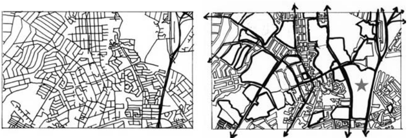
7.5 The impact of neighbourhood closures on the broader environment in northern Johannesburg (including the case-study area, marked with a star), indicating the original street pattern (left) and new urban form (right).
