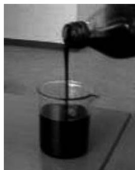
**Fig. 6.3** Bio-oil from flash pyrolysis of biomass pyrolysis
