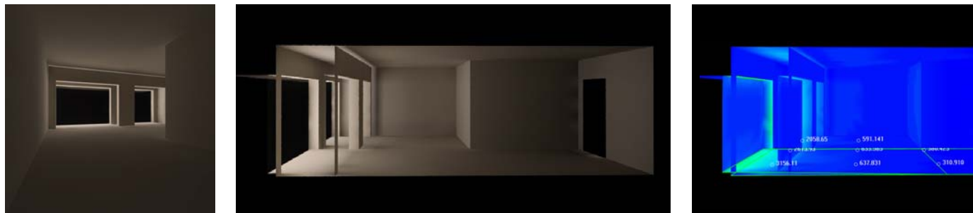
Figure 16 Photo-realistic renderings of 12 PM on 21 June with shading (1 m fixed overhang) showing: (left) view of living room from entry, (middle) section view of south-facing living room, and (right) false-color maps for illuminance that offer a quantitative method for reading renderings. Illuminance levels range from dark blue = 500 lux, light blue = 4,000 lux, green = 8,000 lux, to red = 16,000 lux.
