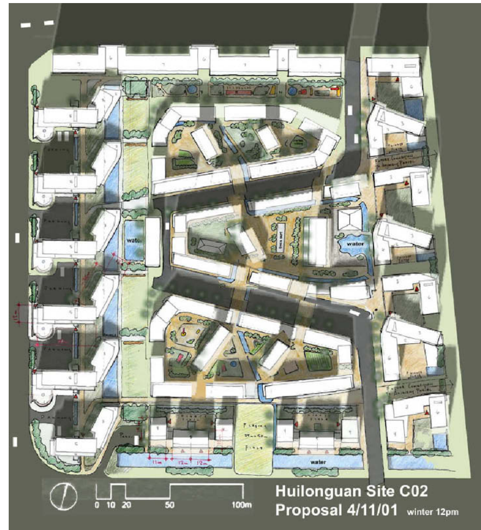
Figure 31b Shading study showing site shadows on 21 December at 12 PM
