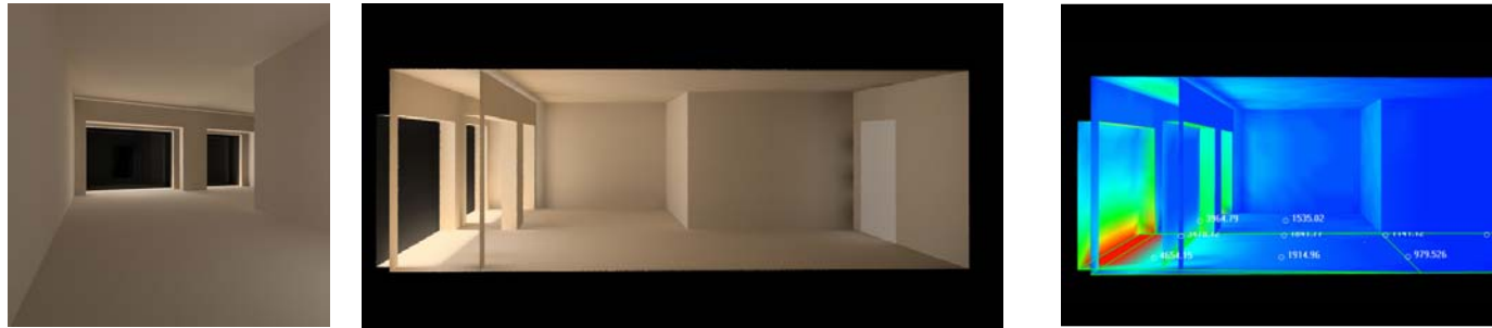
Figure 15 Photo-realistic renderings at 12 PM on 21 June without shading showing: (left) view of living room from entry, (middle) section view of south-facing living room, and (right) false-color maps for illuminance that offer a quantitative method for reading renderings. Illuminance levels range from dark blue = 500 lux, light blue = 4,000 lux, green = 8,000 lux, to red = 16,000 lux.
