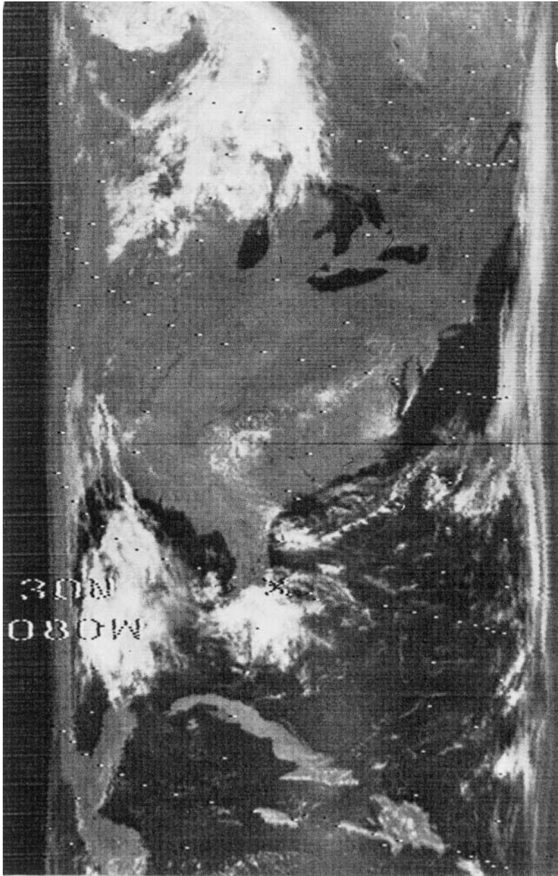
Fig. 5.4.11 Example of the continuous image strip generated by the High Resolution Infrared Radiometer on Nimbus 1. The east coast of North America is in the center. Strong distortion towards the horizons is apparent (Nimbus Project, NASA).
