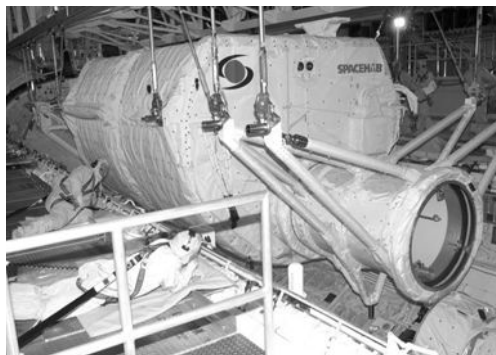
The Spacehab Module and FREESTAR are installed in Columbia's cargo bay on May 24, 2002.
