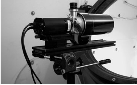
The Kirtland setup with a laboratory CCD camera pointed at a 3.5-inch telescope and a computer-controlled mirror. Photo courtesy of Kirtland AFB.
