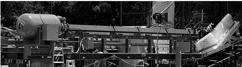
The compressed-gas "chicken gun" used to fire foam blocks at a simulated shuttle wing.
