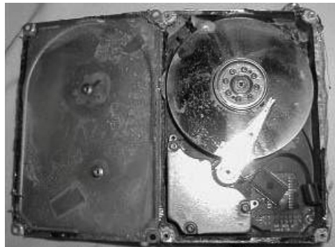
The CVX hard drive was found but heavily damaged. A commercial company which retrieves data from hard drives was able to recover most of the lost data. Photo courtesy of Dr. Robert Berg.
