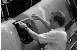
Engineer Dan Bell measures the hole created by the 1.67-pound foam block traveling at 500 m.p.h.
