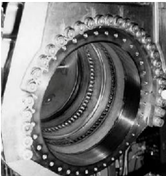
A closeup view of Columbia's flowliners in the 17-inch wide propellant lines. Photo from the author's collection.
