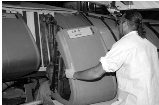
A typical installation of a Reinforced Carbon-Carbon panel on the leading edge of a shuttle's wing.
