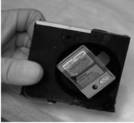
One of the off-the-shelf HOBO temperature recorders that survived the accident and continued to work.
