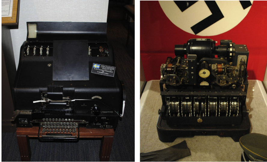
Fig. 5: The Geheimschreiber and the Lorenz machine suffered from similar weaknesses as the Enigma. The Germans used them anyway, and their enemies in World War II broke them.
