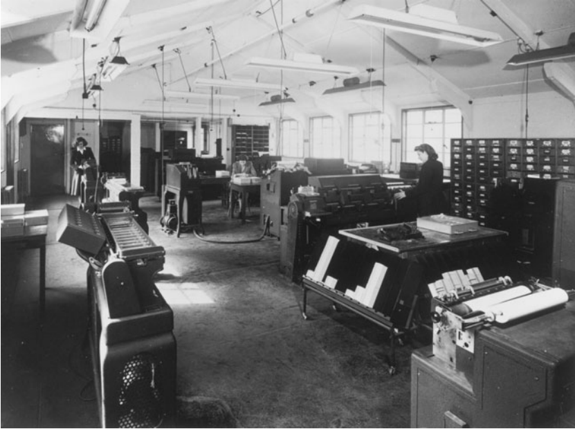
The Hollerith Room in the Babbage Building at the NPL. Turing adopted Hollerith punched-card equipment to provide input/output for the ACE.
