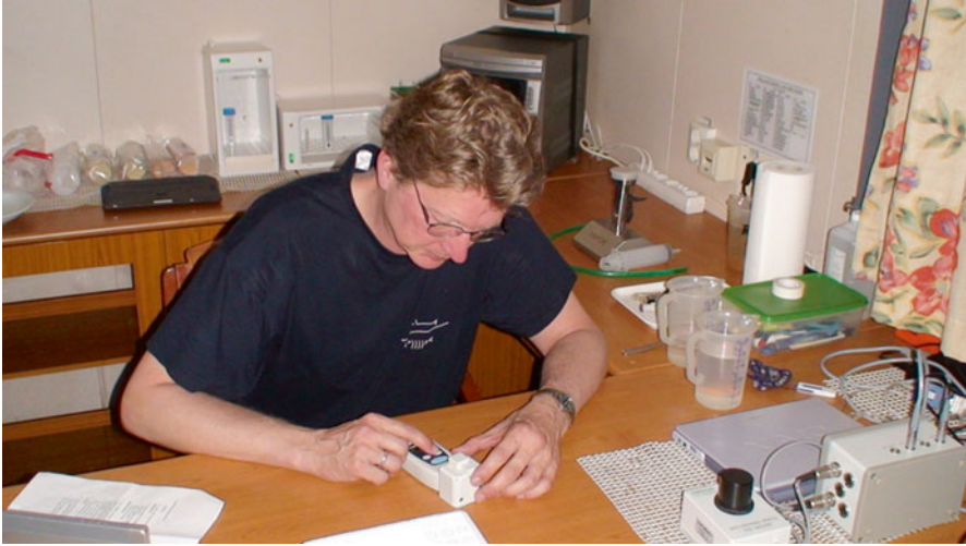
Fig. 23 Hand-held fluorometer used on board
