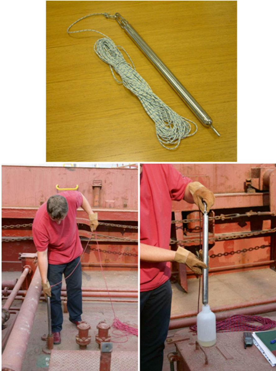
Fig. 8 Point-source sampler used for sampling ballast water through sounding pipes
