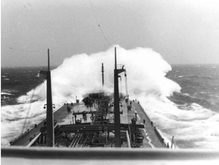
Fig. 14 Vessel in heavy weather conditions, waves in longitudinal effect (Source: Cornelius de Keyzer, Master Mariner, Port of Rotterdam, the Netherlands)
