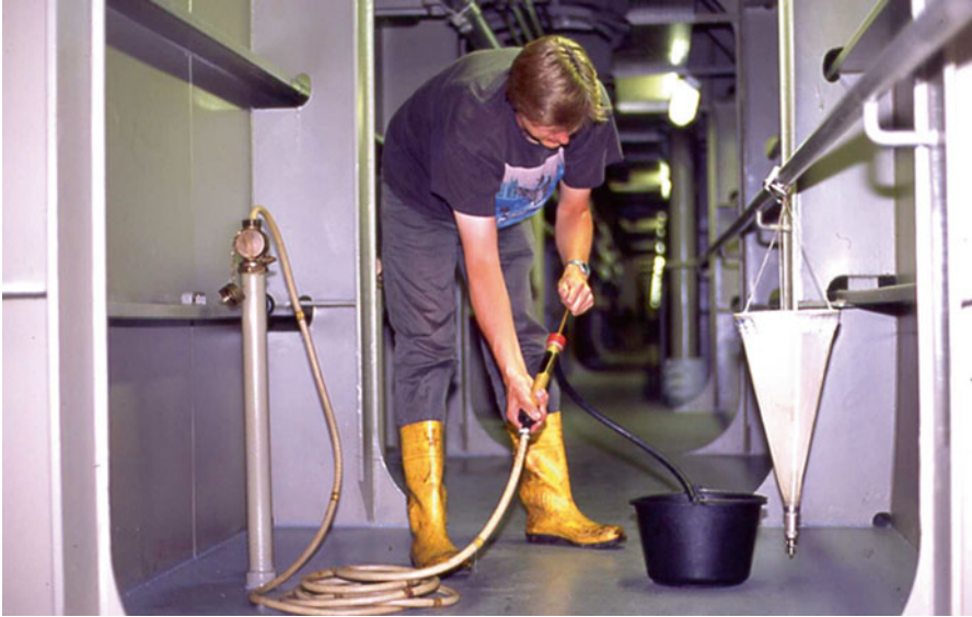
Fig. 10 Hand pump in operation during ballast water sampling
