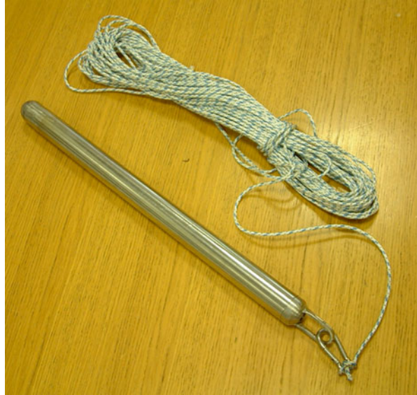
Fig. 7 Water column sampler suitable for ballast water sampling via sounding pipes
