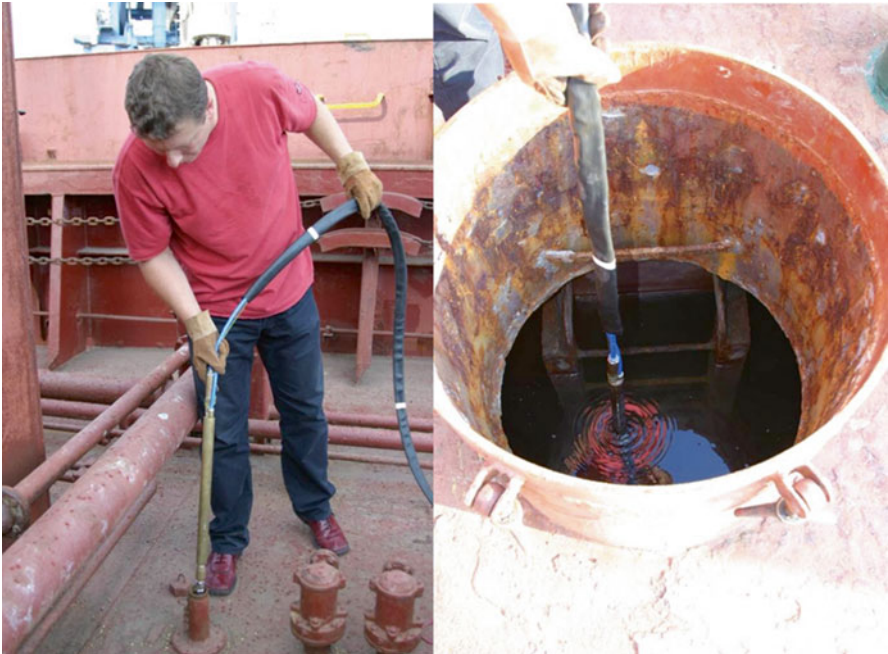
Fig. 11 Air-driven well pump used for sampling via sounding pipe or manhole/tank hatch
