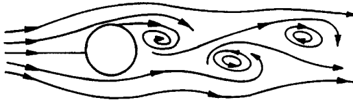
Figure 3.13 Karman vortices behind a cylinder.
