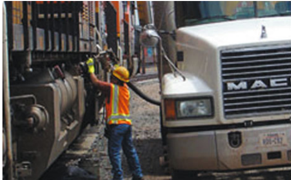
Fig. 2.2 A locomotive being refueled by a fueling truck (Source: http://www.locomotiveservice.com/index.php )
