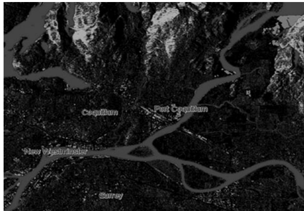
Fig. 21.2 RADARSAT-2 image (in grayscale) showing flooding along the Fraser River, New Westminster and Port Coquitlam area, BC, Canada. 1 ©Canadian Space Agency, 2014. The original color version of this can be viewed at http://www.asc-csa.gc.ca/images/satellites/radarsat2/image-vedette/amerique-nord-coquitlam.jpg
