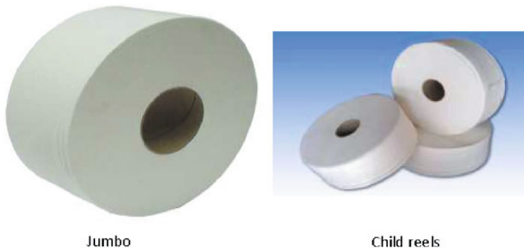
Fig. 17.1 The big Jumbo is slit into child reels of required widths
