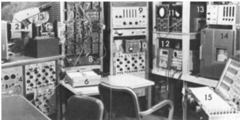
FIG. 1-21. A modern EEG and perceptual laboratory, equipped for EEG, average evoked potential, and CNV recording. 1. Tektronix 502 oscilloscope; 2. Tektronix Polaroid camera; 3. Grass Kymograph camera; 4. Grass physiological stimulators; 5. Tektronix power supply, waveform and pulse generators; 6. Moseley X-Y plotter; 7. Massey-Dickinson control and programming equipment; 8. Power supply; 9. Hewlett-Packard counter; 10. Tapereader; 11. Oscilloscope monitors; 12. Mnemotron computer of average transient (CAT) and accessories; 13. Preset controller and tape coder; 14. Ampex FR-1300 7-channel FM tape recorder; 15. Grass Model 6 8-channel EEG.
