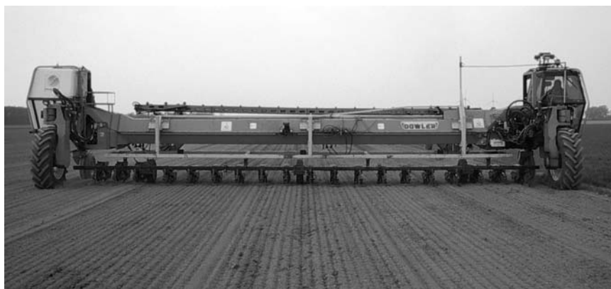
Fig. 8.1 Dowler gantry with a track width of 12 m (Source: Experimental Farm Oostwaardhoeve, Sluutdorp, the Netherlands)
