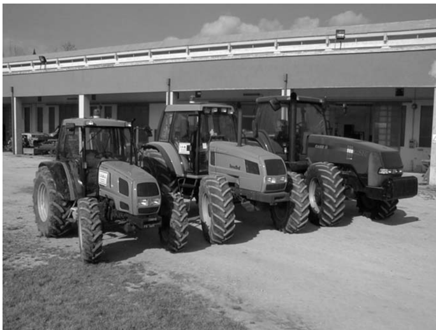
Fig. 10.6 Instrumented tractors of three different power classes
