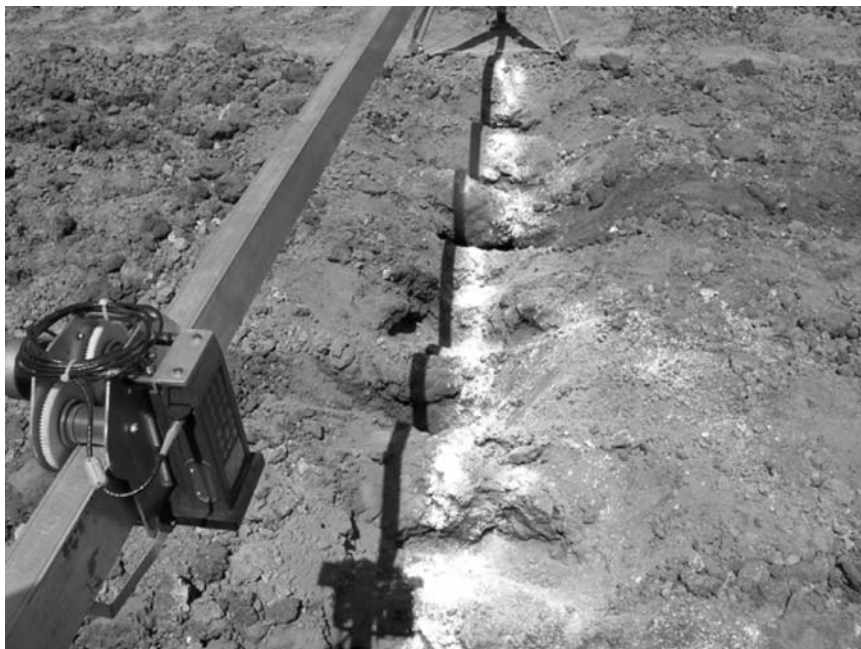
Fig. 10.1 Laser microreliefmeter used for determining the surface roughness before and after the tillage, the tillage depth and the uniformity of the tillage bottom
