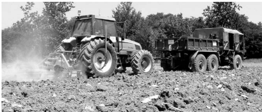
Fig. 10.3 Dynamometric vehicle during traction tests with a three-furrow plough
