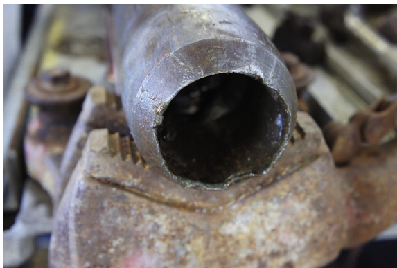
Figure 4 A cutting shoe of a hydraulic piston corer. The front edge is bent and damaged from hitting harder material. Photo: Kallmeyer, GFZ Potsdam.
