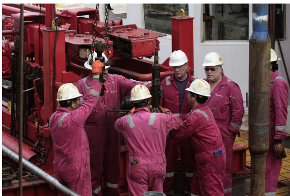
Figure 5 A wireline corer is about to be deployed onboard JOIDES Resolution. The spearhead sits on top of the corer, and the overshot assembly is hanging on chains at the left. A piece of drill string can be seen in the foreground on the right. Photo: Kallmeyer, GFZ Potsdam.
