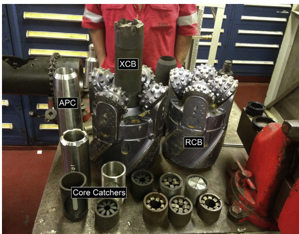
Figure 3 A selection of drill bits and core catchers used on the Integrated Ocean Discovery Program drill ship JOIDES Resolution. Photo: Anna Ling, University of Miami.
