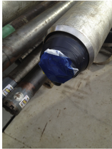
Figure 8 A small plastic bag filled with microsphere tracer solution taped at the bottom of a piston corer. The bag will burst open when the corer hits the sediment and release the microspheres that will bathe the core in a highly concentrated tracer solution. Photo: Kallmeyer, GFZ Potsdam.
