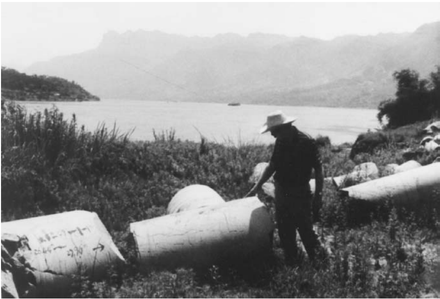
FIGURE 2.8 Large diameter rock samples at the Three Gorges Dam, China.
