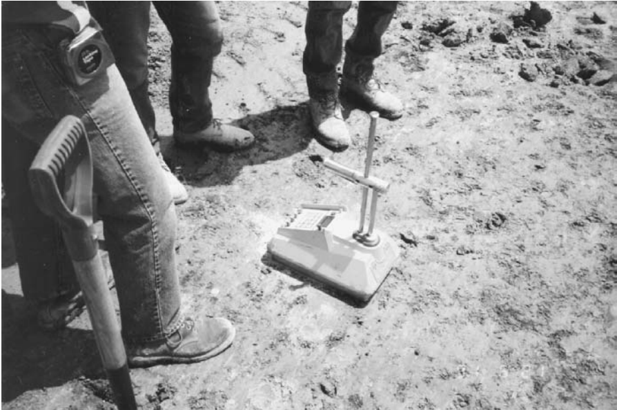
FIGURE 9.4 Nuclear density test.
