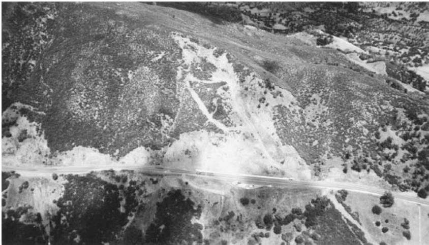
FIGURE 14.10 Typical landslide along a highway cut area.
