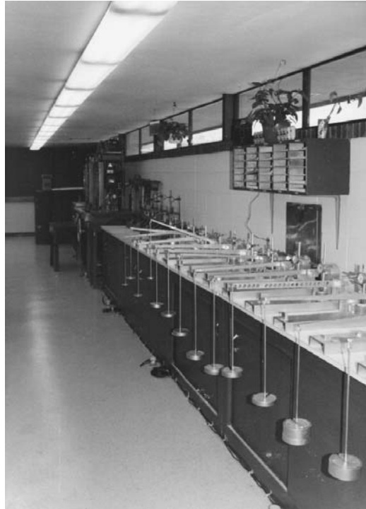
FIGURE 5.2 Modified Consolidation Test.
