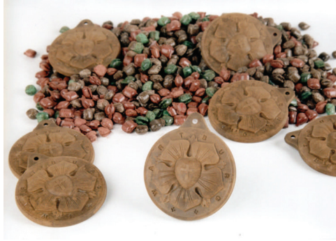
Figure 5.4 Granules of a lignin-based composite and injection moulded sample. (© Tecnar GmbH, 2013.)
