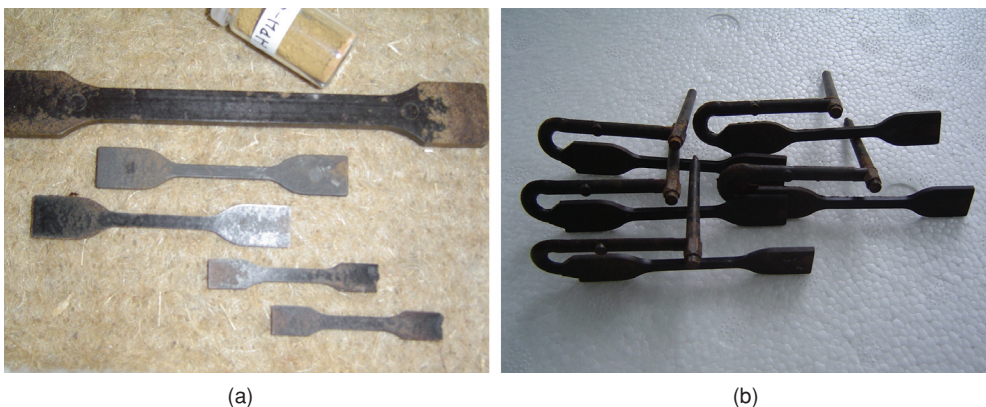
Figure 5.15 HPH-lignin and test material samples composed of HPH-lignin, natural fibres and natural additives obtained by injection moulding. (© Fraunhofer ICT, 2013.)
