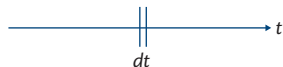
Fig. 5.18.3 The fundamental diagram of dynamical modelling in continuous time. By focusing on what happens during a small interval of time, between t and t + dt , we are enabled to derive differential equations whose solution will describe how the system evolves over time.
