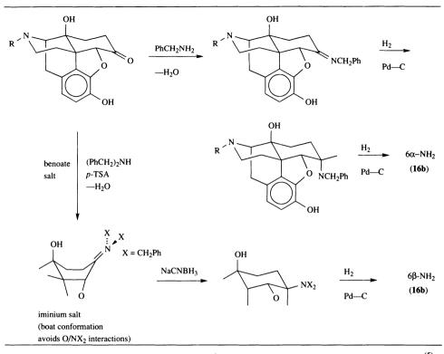
Scheme 13.2. Stereospecific synthesis of  $6\alpha$ - and  $6\beta$ -naltrexamine (R = CH<sub>2</sub>c--C<sub>3</sub>H<sub>5</sub> in formulas shown.<sup>(5)</sup>
