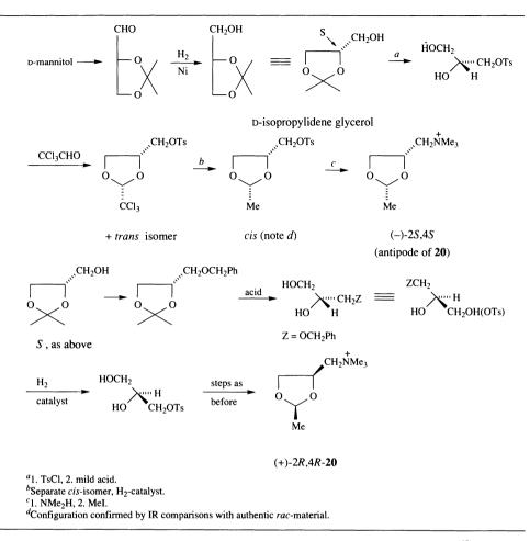
Scheme 8.7. Stereospecific synthesis of antipodes of the dioxolane 20 from D-mannitol.<sup>(48)</sup>
