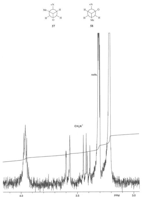
**FIGURE 8.2.** Part of the 400-MHz <sup>1</sup>H-NMR spectrum of *rac*-muscarine chloride (1 mg in CD<sub>3</sub>OD, 130 scans). The methylene proton signals of the  $CH_2^+NMe_3$  side chain appear near 3.58 and 3.42 ppm, respectively.
