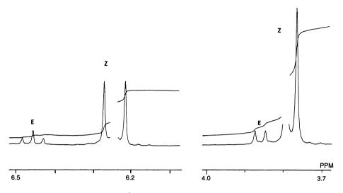
**FIGURE 11.4.** Part of the 270-MHz <sup>1</sup>H-NMR spectrum of the Z-isomer of triprolidine HCl in  $D_2O$  containing the *E*-isomer as contaminant. The triplet pair between 6.2 and 6.5 ppm is due to the vinylic protons (*E* 6.46, *Z* 6.24 ppm) and the doublet pair near 3.8 ppm to the methylene protons adjacent to nitrogen (*E* 3.86, *Z* 3.78 ppm). Pure isomers displayed single-triplet and single-doublet signals (after Granellin *et al.*<sup>(13)</sup> and Granellin<sup>(21)</sup>).
