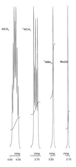
**FIGURE 8.1.** Part of the 400-MHz <sup>1</sup>H-NMR spectrum of acetylcholine chloride in  $D_2O$  at 20° C. The OCH<sub>2</sub> methylene multiplet (lower field near 4.57 ppm) is more complex than that of the <sup>+</sup>NCH<sub>2</sub> signal (near 3.76 ppm) as a result of coupling between <sup>14</sup>N and the  $\beta$ -protons. The spectrum remains second order in spite of being run at 400 MHz; the original analysis was based on 60-MHz data.<sup>(89)</sup>
